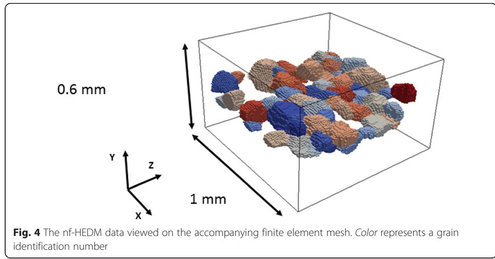
represented to within the resolution of the finite element mesh. This shows the distinct difference in grain shape when using the full field morphology from the nf-HEDM data.
