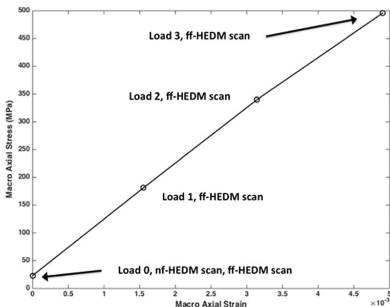
**Fig. 2** Macroscopic stress-strain curve for the HEDM experiment. The sample was held at load 0, load 1, load 2, and load 3 in order to take ff-HEDM measurements. Note that a slight non-linearity appears to develop between load 2 and load 3
