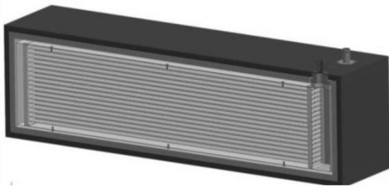
Figure 2. GEN-I Radiator-Type PCM Thermal Storage Module
