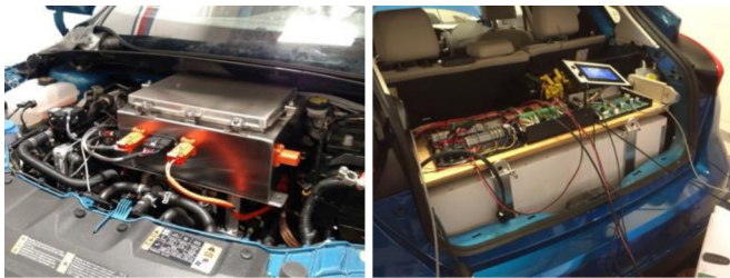
Figure 7. Retrofitted EV with PCM Thermal Storage System
