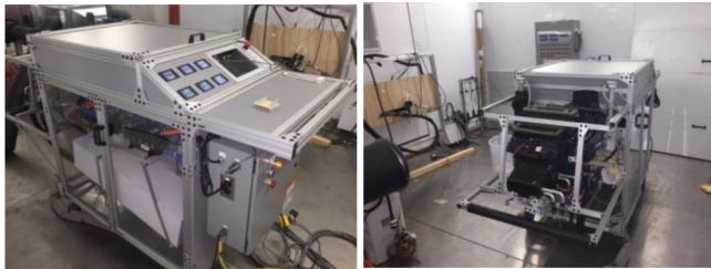
Figure 5. Photos of the ePATHS Bench Prototype Hardware in ORNL's BTRIC Test Chamber
