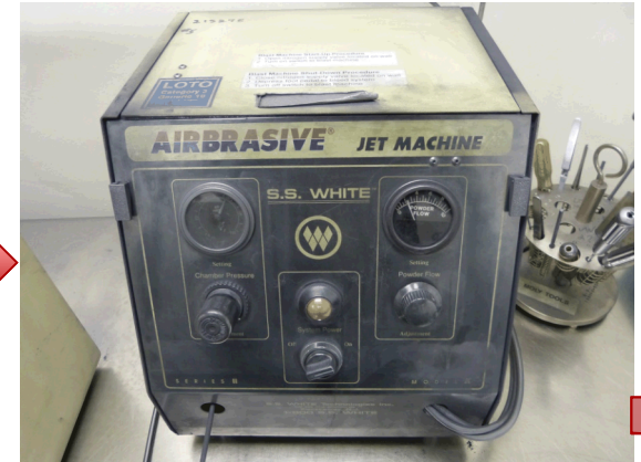
Load MoS 2 in Powder Feeder
