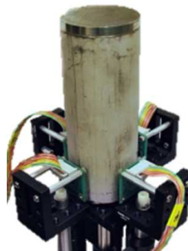
Sensing temperature through stainless steel tube
