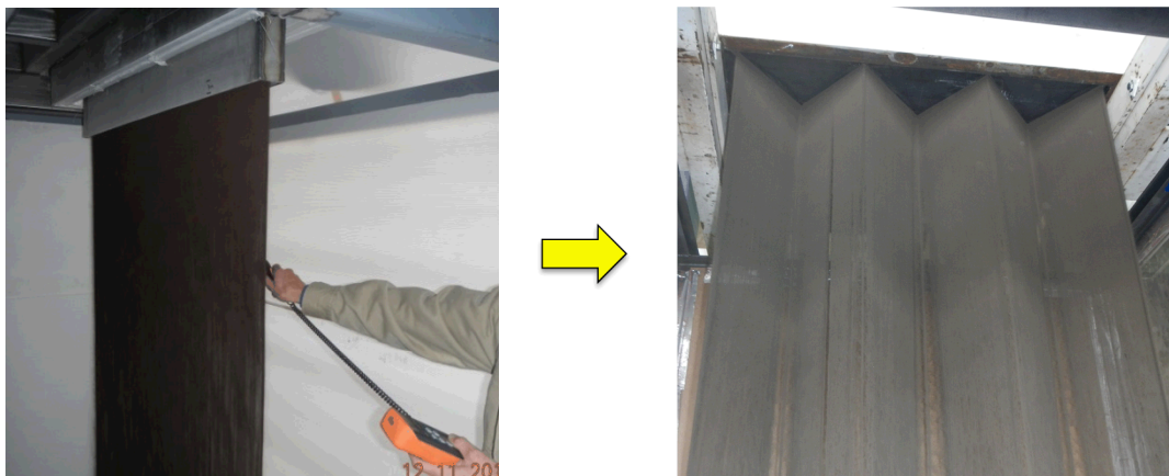
Figure 1. Images of conventional straight-line (left) and new zig-zag (right) particle release patterns for falling particle receivers.
