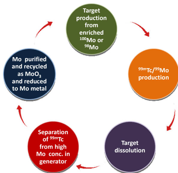
Figure 1 Diagram of molybdenum cycle from the disk production through the recycle process
