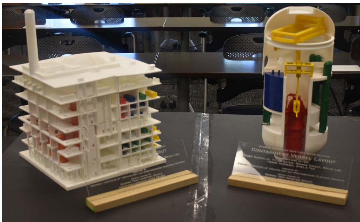
Figure 4.7. 3D models of the reactor vessel, nuclear island and containment
