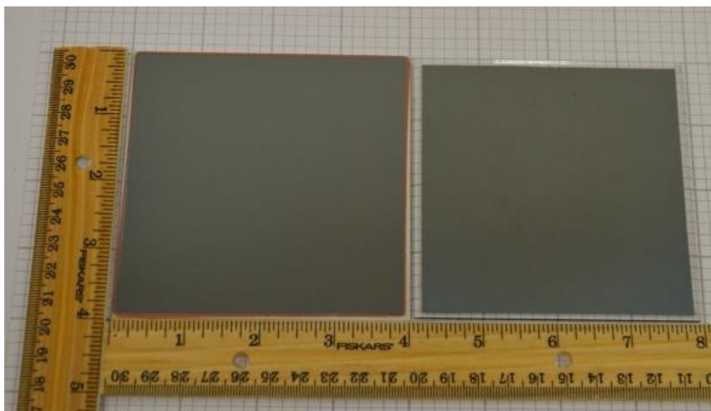
Figure 18. Enriched ^{10}\text{B} -doped a-Se (As, Cl) thin films with \sim 450 \mu\text{m} thickness deposited on 10 \times 10 \text{ cm}^2 ( 4 \times 4 sq. inches) substrates: (left) Al/ \text{Al}_2\text{O}_3 substrate and (right) ITO coated glass substrate.
