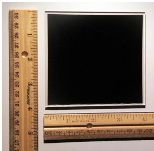
Figure 19. Lithium-doped a-Se alloy films (525 \mu\text{m} thickness) on 10 x 10 \text{cm}^2 (4x4 sq. inches) ITO coated glass substrates.
