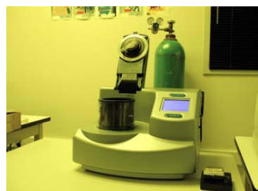
RF/DC 13.56 MHz frequency sputtering unit
