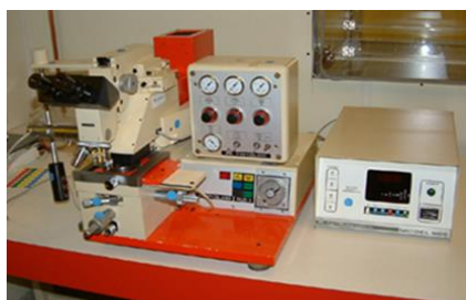
Photolithography: Karl Suss model MJB 3 Mask Aligner, Min. pitch size: 0.5 \mu\text{m}
