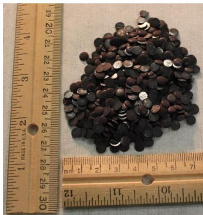
Figure 12. Dry pellets of ^{10}\text{B} -doped (32 a/o) a-Se (0.52% As, 5ppm Cl) alloy material.
