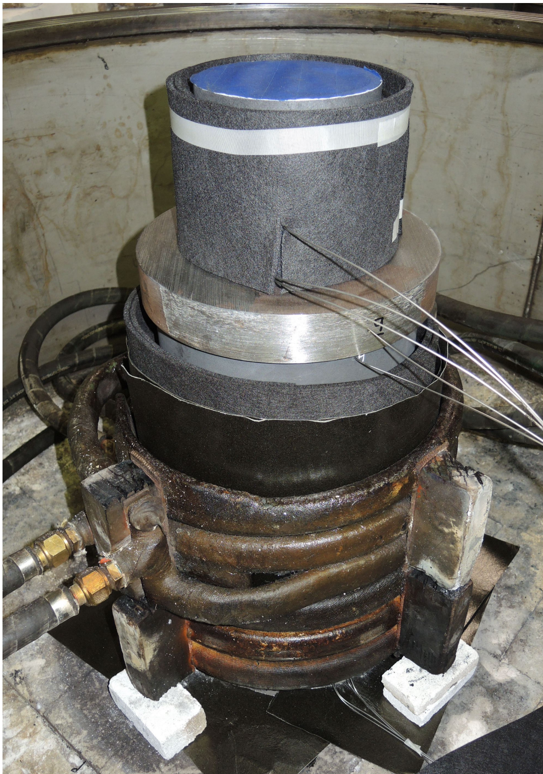
Fig. 39 Counter gravity casting mold assembly prior to installation of the induction heating coils and insulation. The stainless steel sheathed type-K thermocouples are the silver wires. Blue painters tape keeps mold interior clean during assembly and is removed prior to casting 17K-696.
