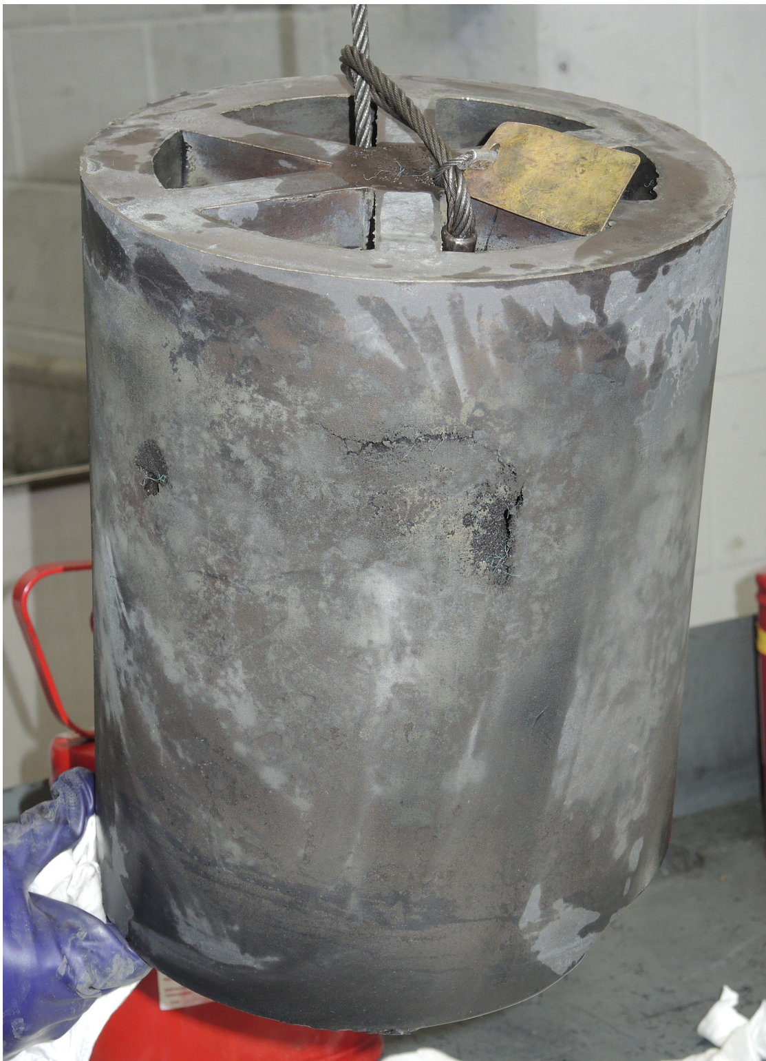
Fig. 44 Resulting casting 17K-698 from counter gravity 250 mm with revision C mold. Casting is show upside down with bottom of casting at top of photo.
