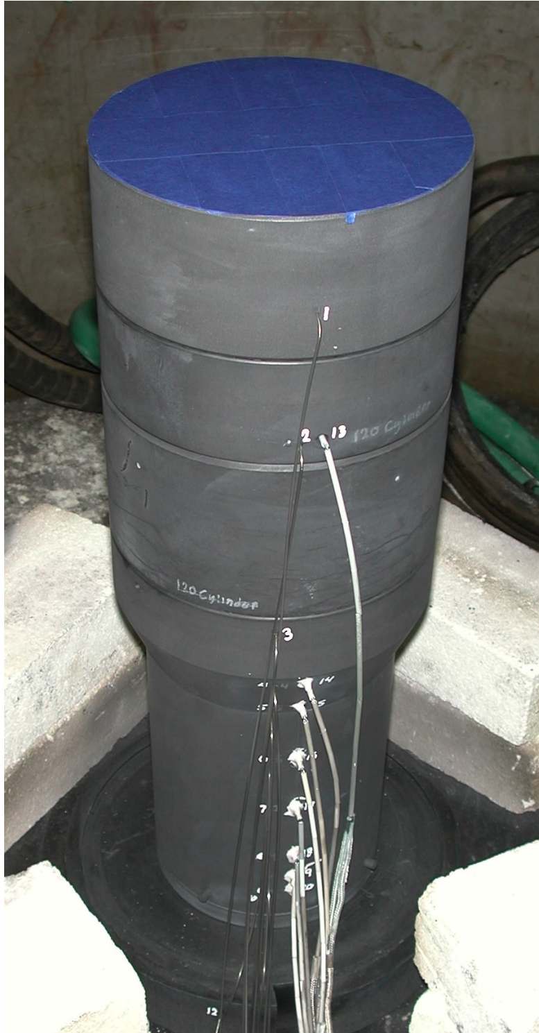
Fig. 6 Top fill casting mold assembly prior to installation of the induction heating coils and insulation. The stainless steel sheathed type-K thermocouples are the silver wires while the alumina sheathed type-C thermocouples are the segmented white strands. Blue painters tape keeps mold interior clean during assembly and is removed prior to casting.
