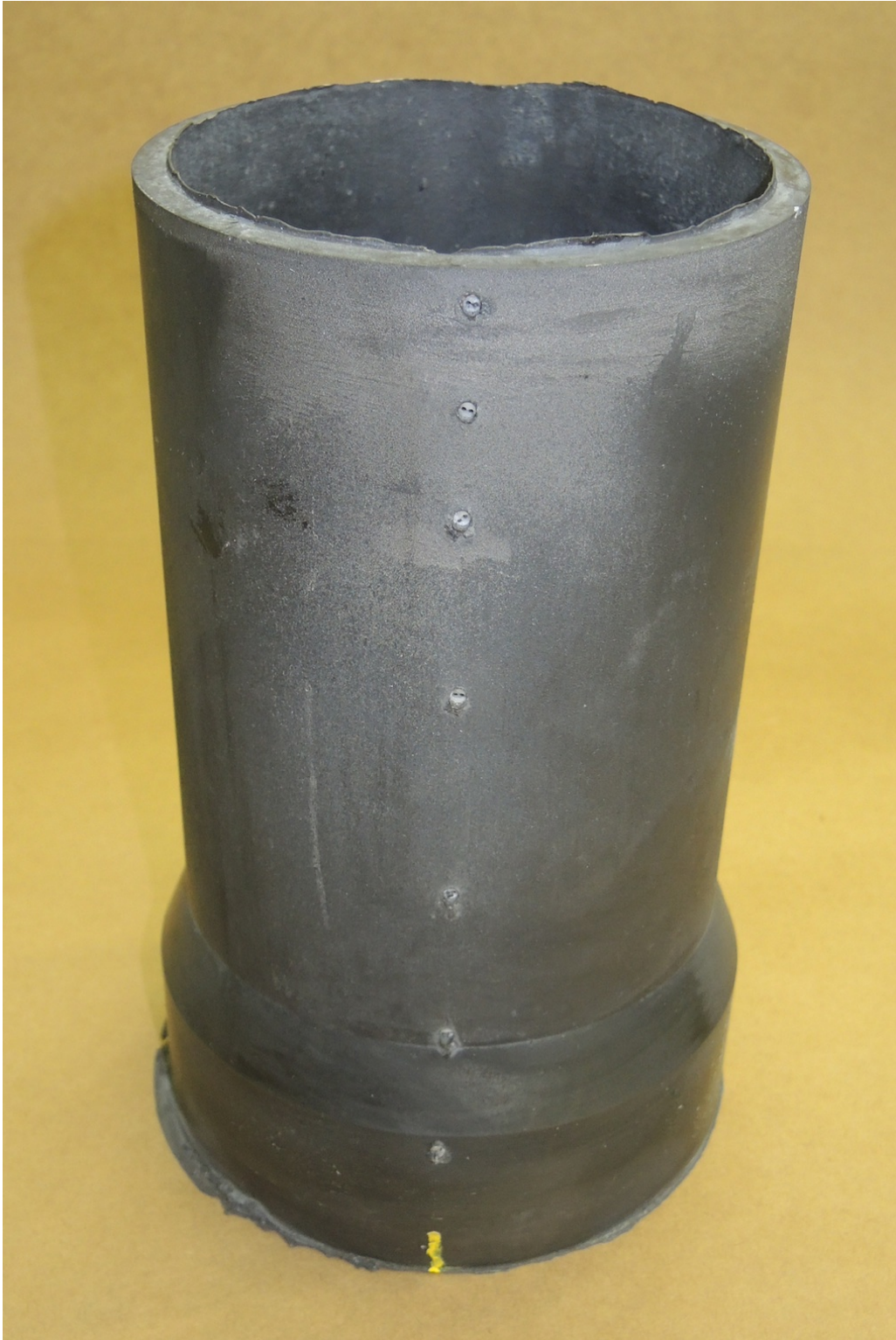
Fig. 15 Photograph of the counter gravity 120 mm cylinder casting in the as-cast state. The graphite core is still in the casting and tips of the type-C thermocouples are imbedded in the metal.
