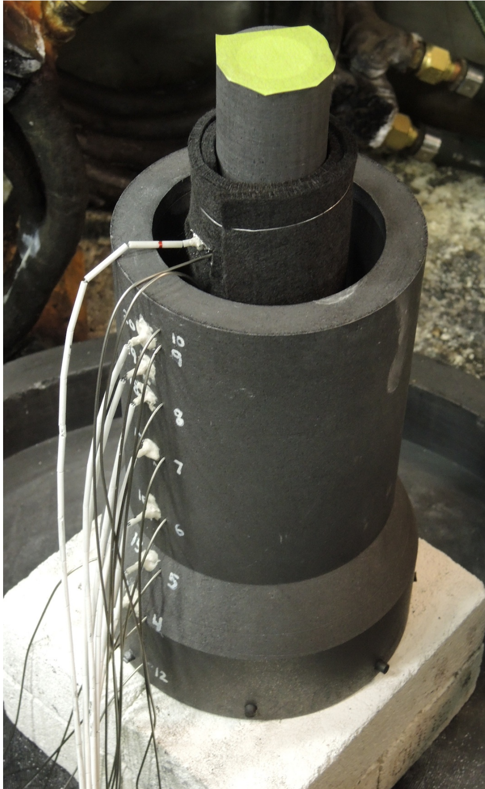
Fig. 9 Counter gravity casting mold assembly prior to installation of the induction heating coils and insulation. The stainless steel sheathed type-K thermocouples are the silver wires while the alumina sheathed type-C thermocouples are the segmented white strands. Green painters tape keeps mold interior clean during assembly and is removed prior to casting.
