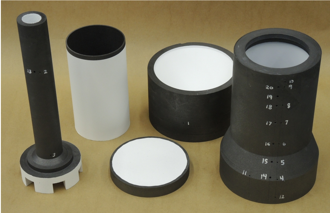
Fig. 7 Mold components of the 120 mm diameter counter gravity mold prior to assembly. The white coating is the yttria mold coating.
