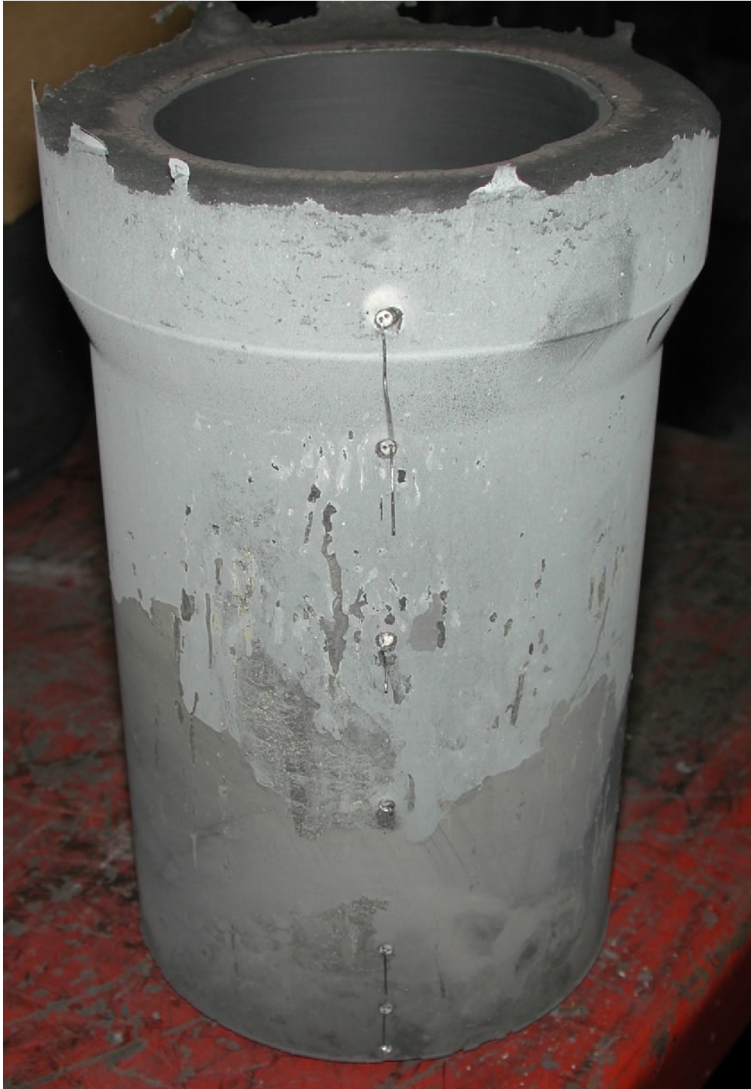
Fig. 14 Photograph of the thin conventional 120 mm cylinder casting, cast at the regular temperature, in the as-cast state. The graphite core is still in the casting and tips of the type-C thermocouples are imbedded in the metal.
