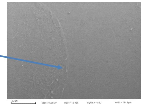
Very few, if any, inclusions are identified and the surface is nearly perfect, in comparison, although several  $\mu\text{m}$ -scale defects are still present
