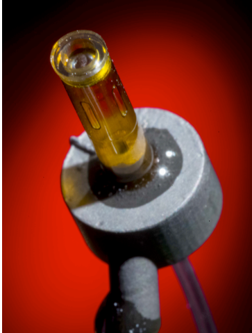
Figure 8: OMEGA-60 MagLIF target, with three azimuthal slits (photo credit: E. Kowaluk)
