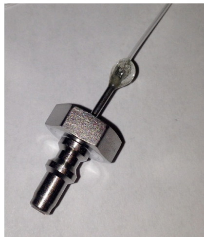
Figure 15: Quick connect fitting for pressure transducer system
