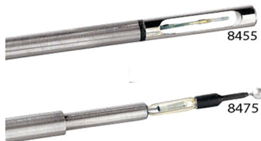
Figure 2.17 Photographs of the two types of hot wire anemometer tips.
