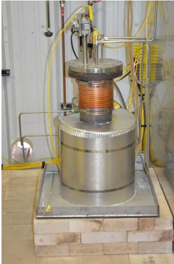
Corrosion studies in molten salt up to 700 C in “salt pots”
