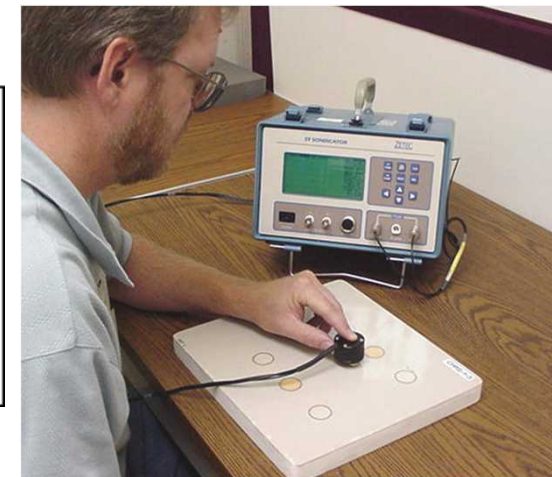
Corrosion Detection with Dual Frequency Eddy Current
