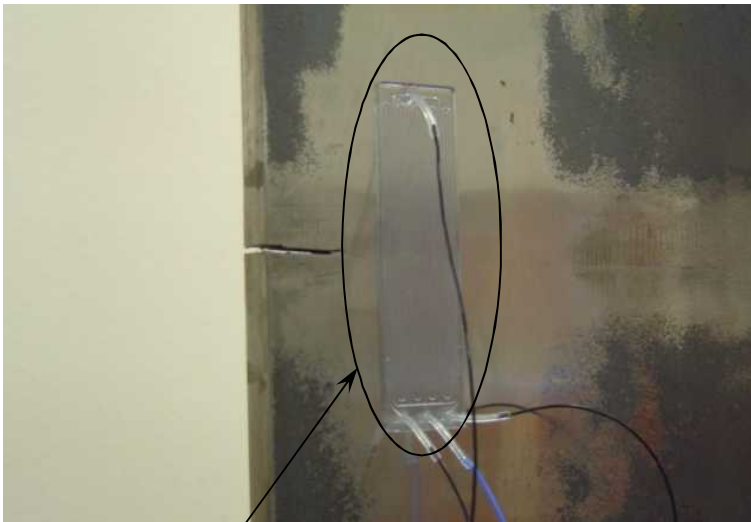
CVM Sensor Adjacent to Crack Initiation Site
