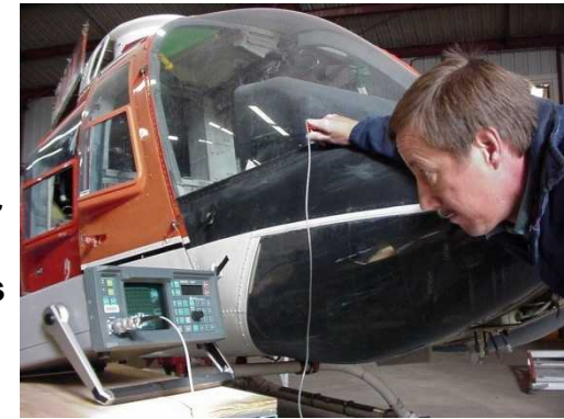
Corrosion Detection with Dual Frequency Eddy Current
