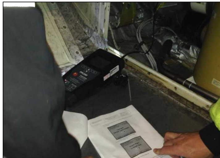
Connecting SLS Leads and Running PM-200 to Monitoring Device to Check Sensor Network
