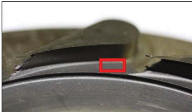
Figure 12.13 Turbine nozzle undercut by erosion at Sandia National Labs (Fleming et al., 2014).
