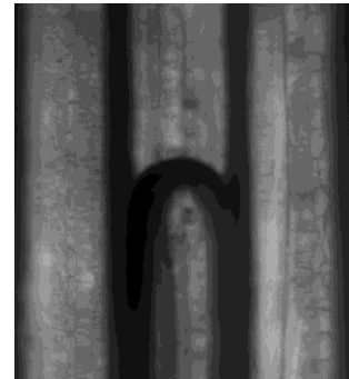
Contact angle measurement Left: non-wetting on printed channel (middle), and wetting contact angle on glass capillary
