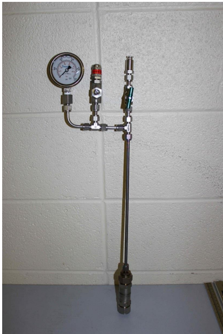
Figure 10. Microreactor used for coal dissolution experiments.
