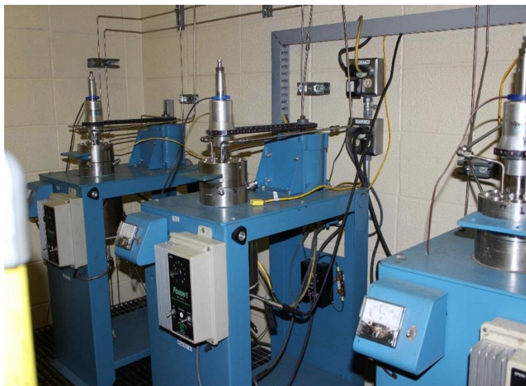
Figure 14. One-liter CSTRs used at PSU.
