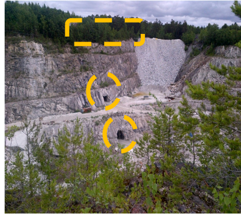
Figure 9. Guidance in selecting sampling sites may be obtained from relational considerations (e.g., proximity to suspected surface ground zero as evidenced by portals or tunnels as shown in circles) and indirect indicators of pathways in shallow soil such as tree roots, especially if indicating damage from ground motion. In the case of evident portals and tunnels, gas sampling should also be performed if accessible.
