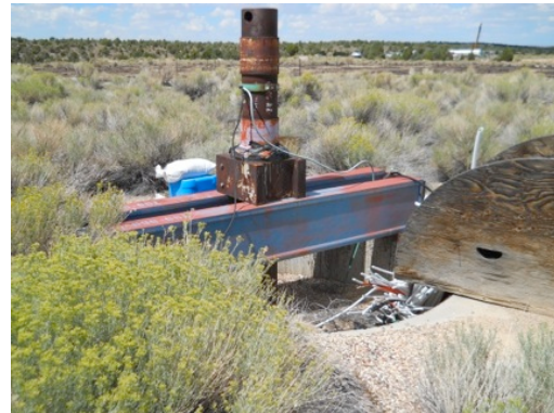
Figure 6. Artifacts or objects associated with a potential UNE site that are connected to the subsurface regime are potentially excellent pathways for gases to reach the surface. Photo is of emplacement casing which has produced detections of gases.
