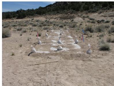
Figure 14. Broad area tarping is appropriate when a tube cannot be easily inserted into a visible surface feature or there is some uncertainty about the location of a feature or pathway.
