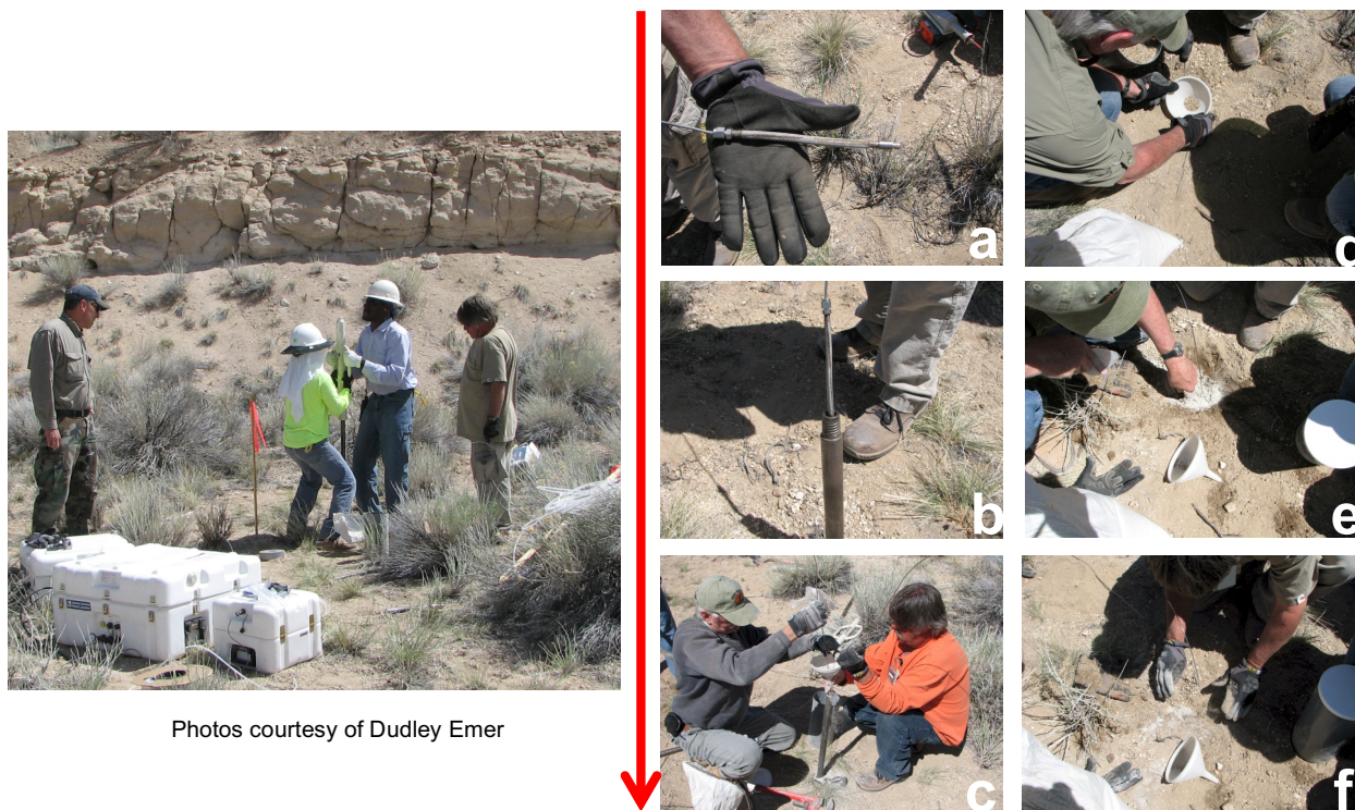
Figure 13. Creating a subsurface sampling point involves several steps. Photographs here illustrate how a subsurface sampling point may be produced. Initially, a hole, several meters deep, was created with a manual Geoprobe ® insertion tool requiring two people to hammer a hollow steel shaft with expendable penetrating point into the subsurface (left). Following insertion of the hollow tube into the subsurface, the series of steps for completing the subsurface gas sampling point are shown on the right (a-f). a) A section of Geoprobe ® pre-packed screen is attached to stainless steel tubing. Screen section allows subsurface gases to be withdrawn from the formation through a sandpack, which will be added between the screen and hole wall. Before inserting the screen a small amount of coarse sand is first dropped into the hollow shaft allowing the screen to rest upon the sand pack. b) The screen connected to the stainless tubing is inserted to the bottom of the hollow shaft. c) More coarse sand is now added through a funnel while moving the tube and screen up and down to prevent bridging of the sand and allow the sand to fill the zone between the hole and screen. Sand is added until the sandpack extends at least a few centimeters above the screen. A tool to estimate sandpack thickness, such as a small diameter rod, may be required. As more sand is slowly added through the shaft hole, the shaft is slowly withdrawn from the hole to allow the sand to fill-in completely between the screen and hole wall. d) Once sandpack is complete, Bentonite clay is
