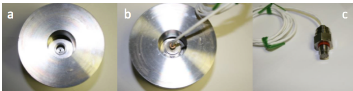
Figure 3. Modification of the top anvil incorporating pressure transducer for P-ODTX: a) top of anvil with bulk head, b) top with pressure transducer inserted, and c) close-up of pressure transducer
