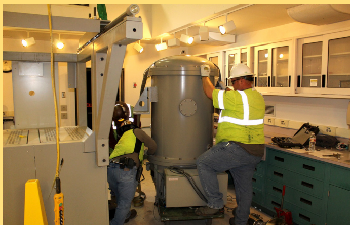
The JEOL 3000 was removed in three large pieces and several smaller pieces. Above, riggers stabilize the microscope's high tension tank on a dolly. To the left of the riggers is the microscope frame that housed the tank, the TEM column, and other components. Below, the TEM column on a dolly outside the Materials Science Laboratory.
