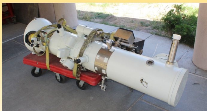
The JEOL 3000 was removed in three large pieces and several smaller pieces. Above, riggers stabilize the microscope's high tension tank on a dolly. To the left of the riggers is the microscope frame that housed the tank, the TEM column, and other components. Below, the TEM column on a dolly outside the Materials Science Laboratory.
