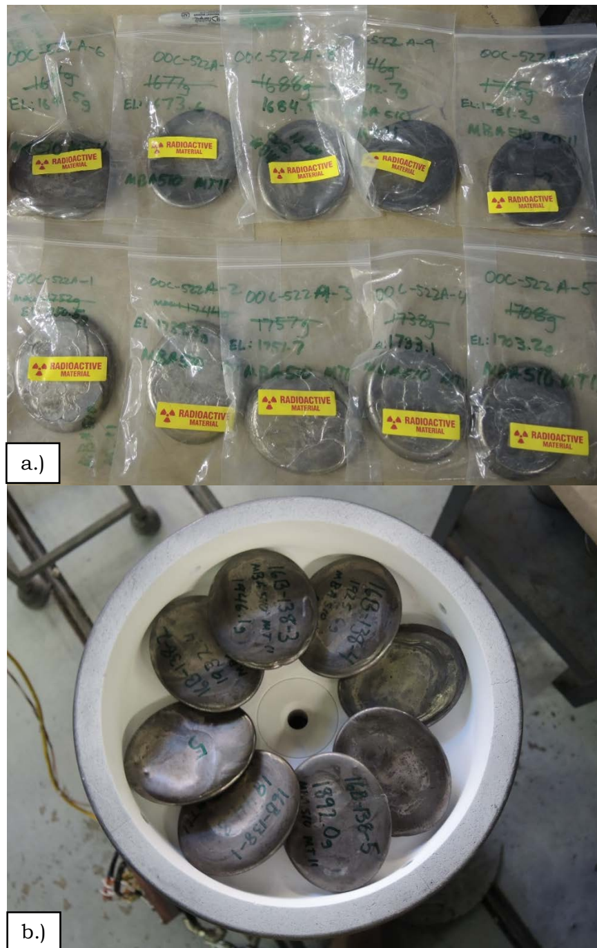
Figure 5: a.) Final buttons from casting IDs 16B-138 and 16B-139. Elemental masses are shown on the sample bags since they were still considered in-process by the time of this photo. b.) The arrangement of the charge material is also presented.
