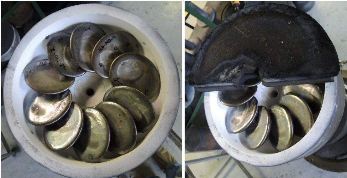
Figure 13: Charge arrangement inside of the crucible (left). Two insulating lids (right) are used as heat shields. The lids are placed on both halves of the crucible, but one half has been removed for clarity.
