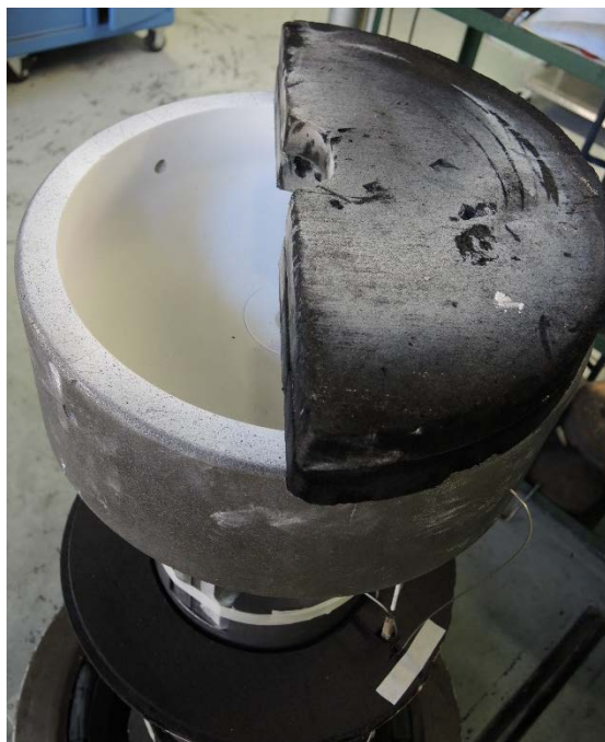
Figure 3: One half of the crucible cover configuration is depicted. The entire crucible is covered during casting. The interior hole is to allow the stopper rod to pass through and leave room for pyrometer measurements near the center of the crucible.
