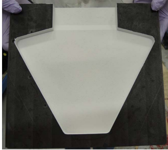
Figure 12: A view of one half of the mold. The interior is coated with a ytria-based suspension with the commercial name of YK.
