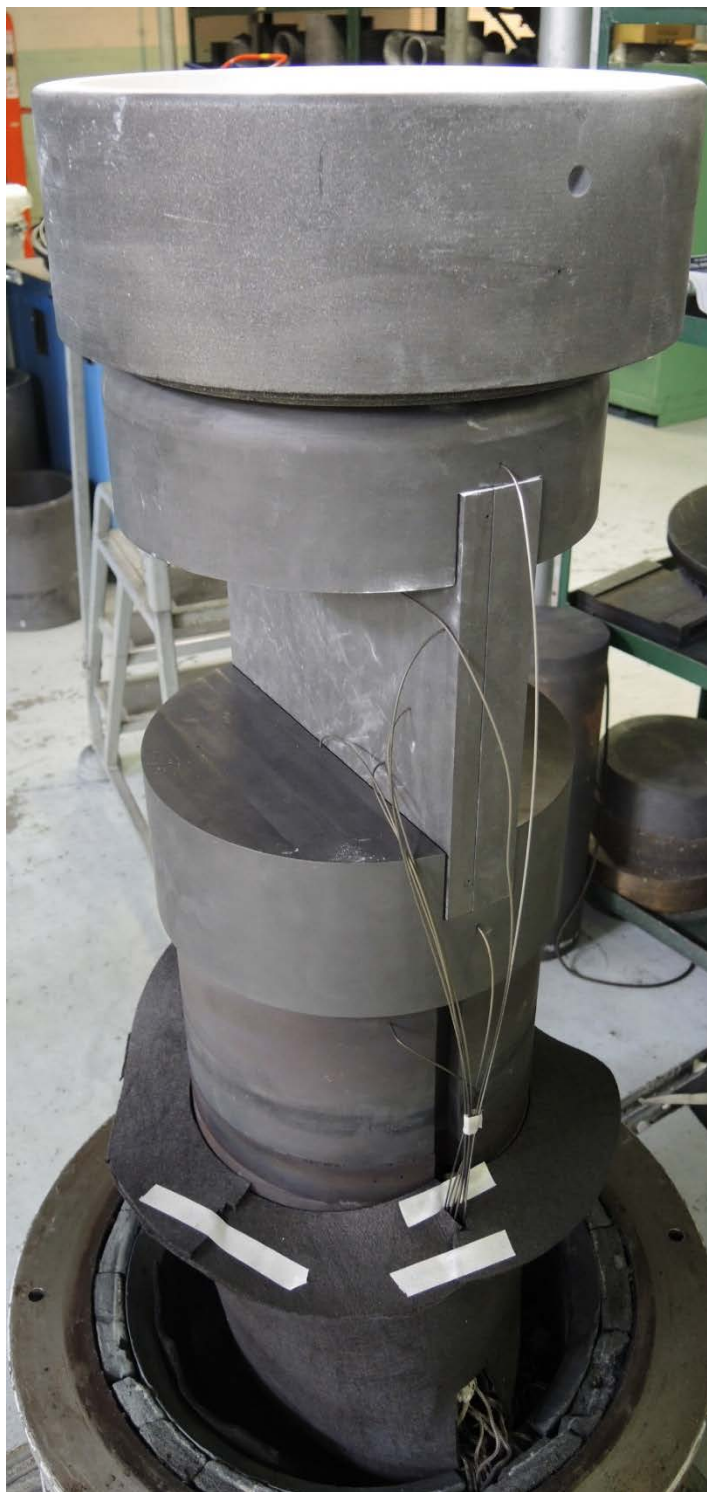
Figure 14: The entire mold stack shown without the insulating lids. Thermocouple placement is evident. Graphite felt was used as a radiative heat shield below the mold to protect the thermocouple feedthroughs and the safety crucible.
