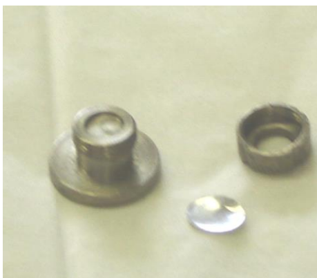
Figure 5. Redesigned target holder for ^{99\text{m}}\text{Tc} production from \text{Mo}_2\text{C} and Mo target material
