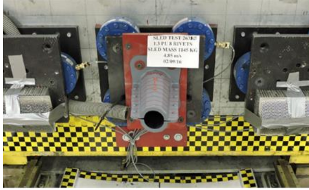
Figure 33. A crush can ready to be impacted on the crash-test sled. Four load cells are used to track the force during the impact. The crush can is mounted stationary on the wall while the sled travels along rails to impact it.
