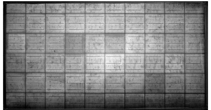
Fig. 7. EL image captured using Method 2 on the fielded panel.
