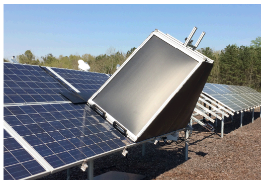
Fig. 1. Hood mounting on a fielded solar panel.
