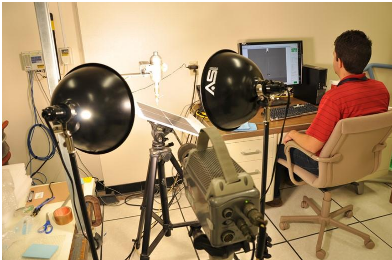
Figure 5. Experimental setup with solar panel, high speed camera, and water dropper.
