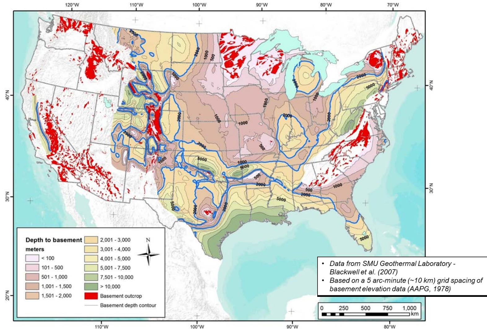
Distribution of crystalline basement at a depth of less than 2 km (tan shading) and granitic outcrop (red) in the contiguous US (from Figure 3-2 in Perry et al., 2015)
