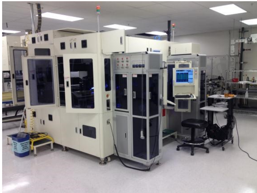
Figure 1.1: Photo of new stringer as installed at Solaria, Fremont HQ (Deliverable 1.1)
