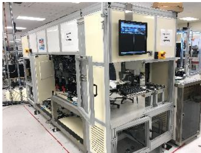
Figure 5.1: Installation of 25MW PowerXT stringer at Solaria HQ
