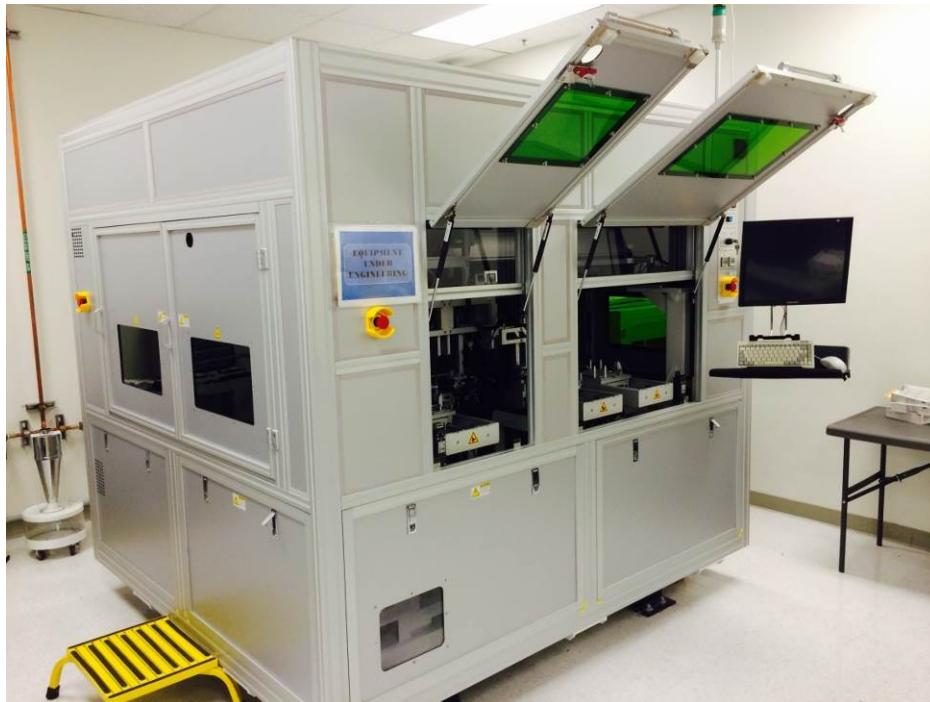
Figure 3.1: Laser scribing machine installed and under testing for compatibility with new singulator and stringer process
