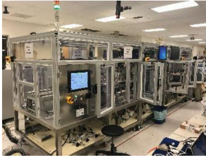
Figure 4.1: Installation of 25MW PowerXT stringer at Solaria HQ
