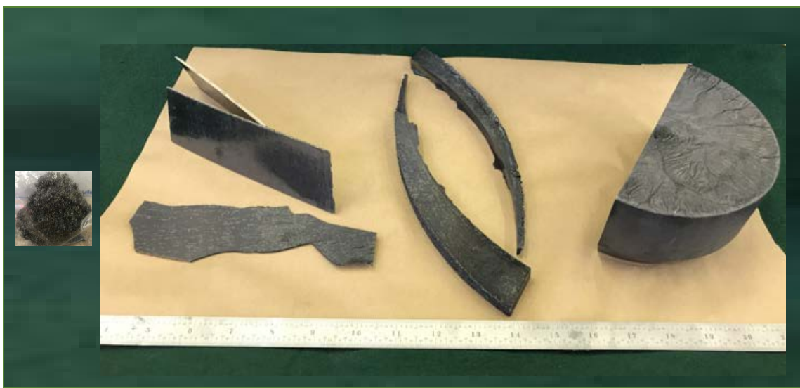
Figure 4: A variety of scrap materials with different shapes and sizes. Working left to right there are bundles of chips, thin rolled plate, thick picture frame, bulk hot tops.
