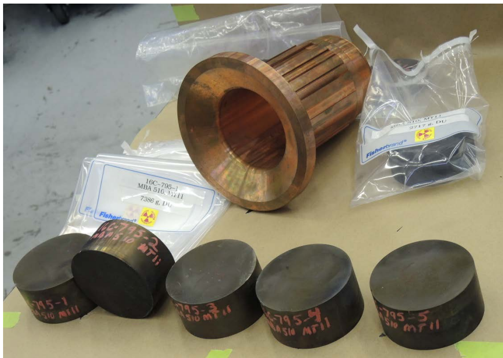
Figure 10: The final machined pucks (foreground) from 16C-795. The PAM water cooled copper crucible can be seen in the background.
