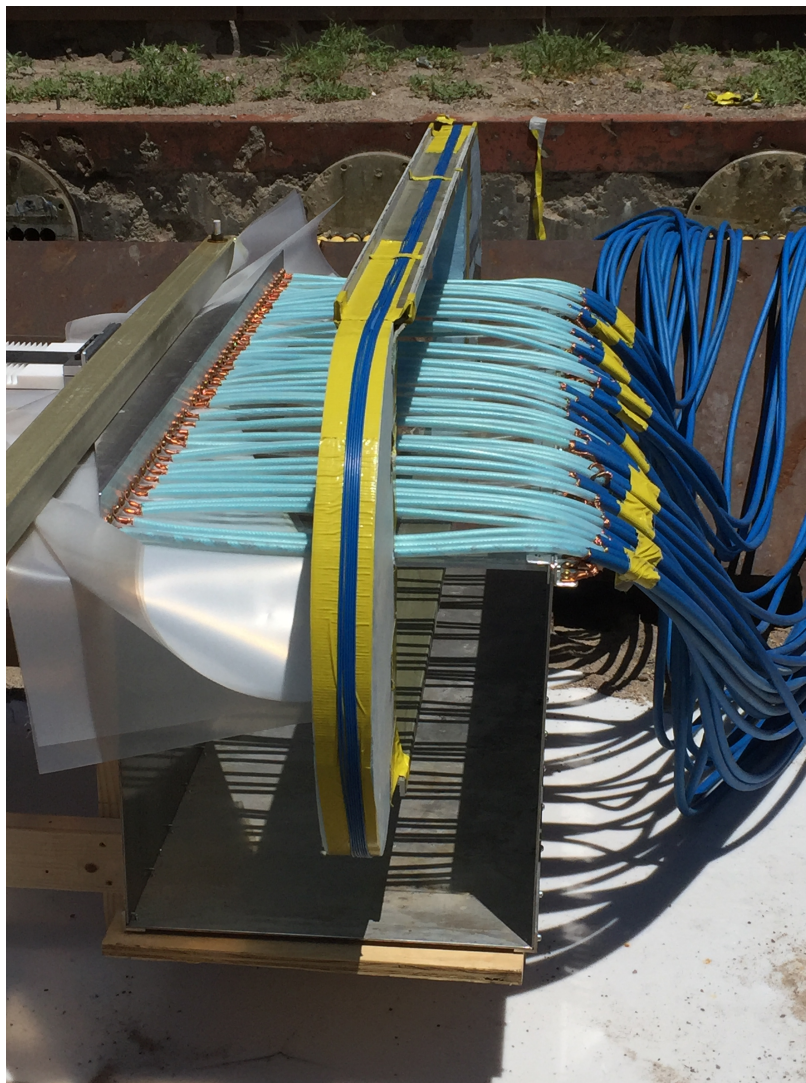
Figure 3.2: Large radiative loop at Point 88 (44 cm on a side), looking along the axis of the loop.
