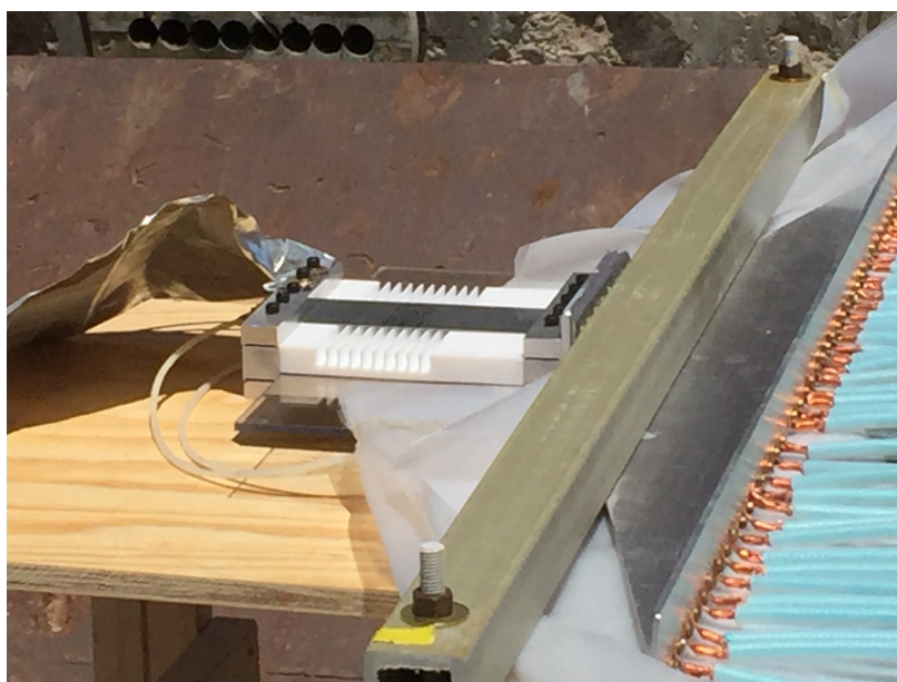
Figure 3.3: EFF (white corrugated former with Invar strip on top at center, with cable attachment assembly to the right).
