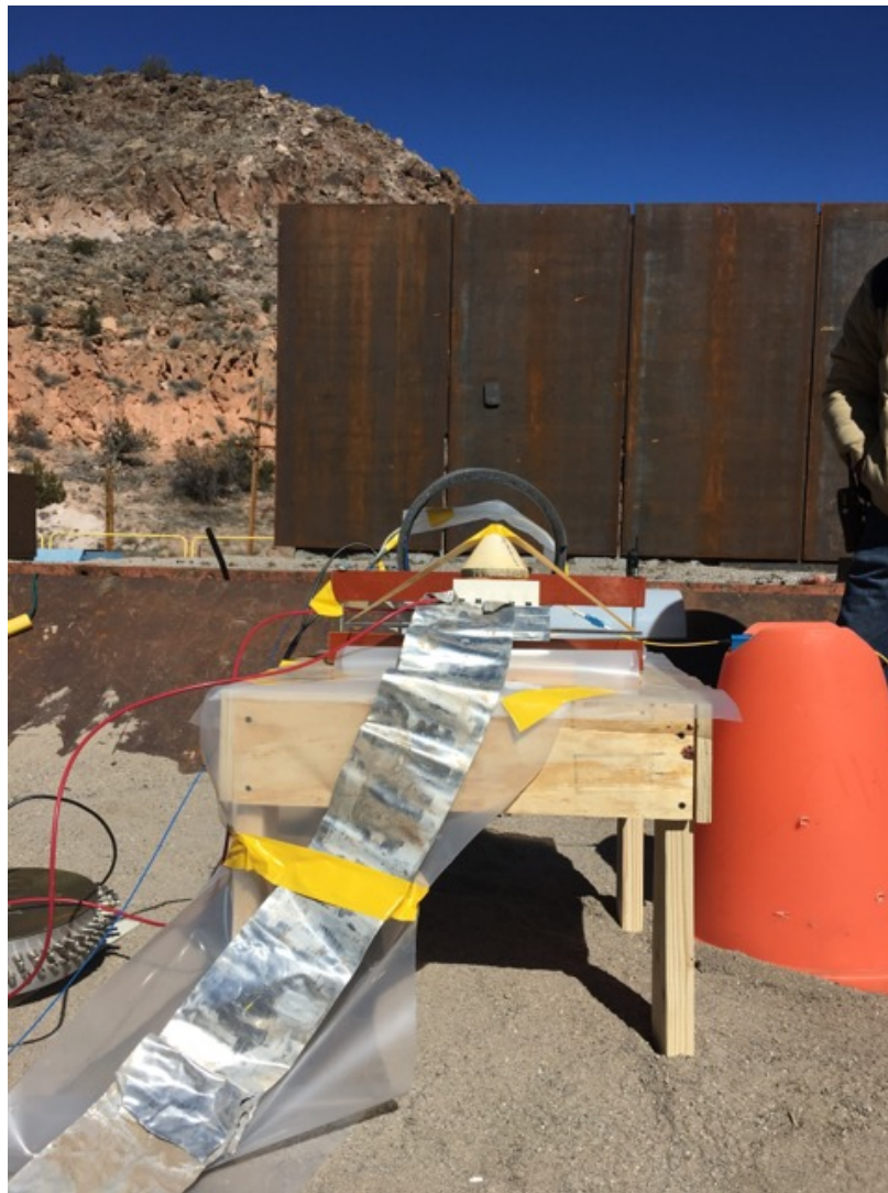
Figure 3.4: The assembled EFF on the firing table. The large metal strip in the foreground is a low inductance connection to the single ground point (out of picture). (Picture from Tim Goorley.)
