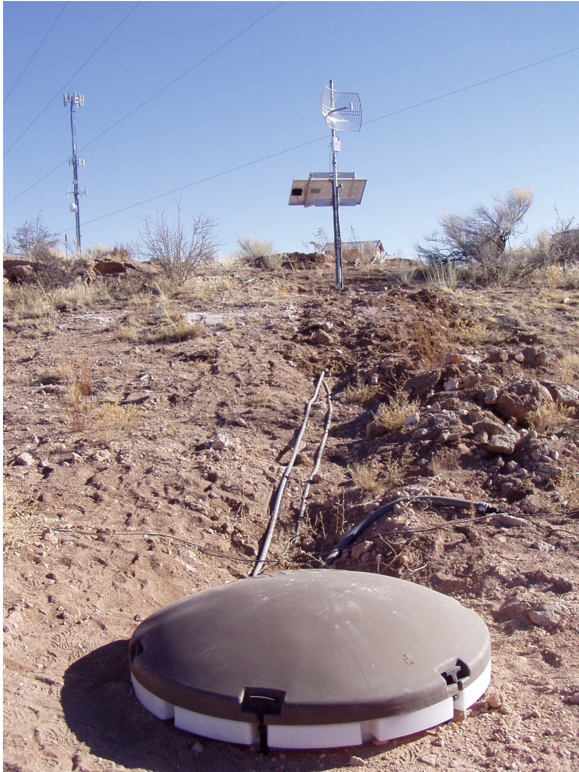
Figure 5: Typical almost-completed LASN broadband seismic station. Seismic vault is in foreground and solar panel/telemetry mast is in background. Electrical conduit connecting them is buried to complete the installation.
