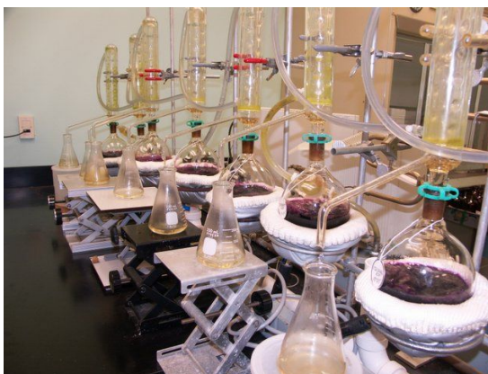
Exhibit 7-2. Distilling Samples for Tritium Analysis Performed at PEARL
