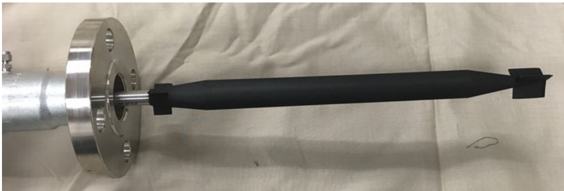
Figure 72: Subsonic ICES 3D Printed Centerbody
