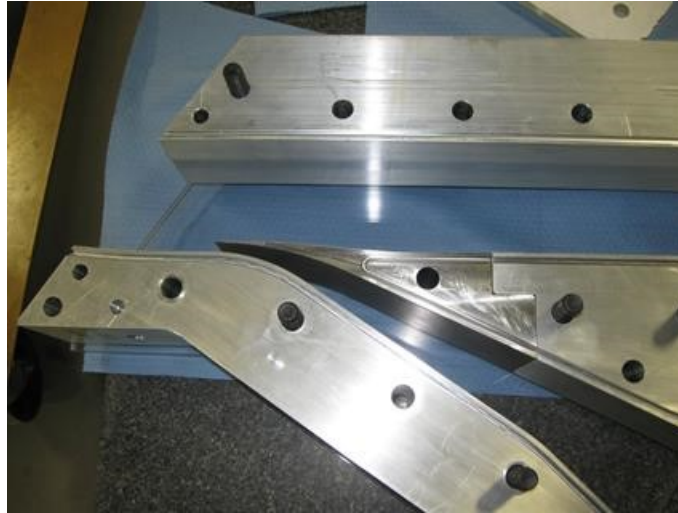
Figure 30. Assembly of the diffuser/capture duct
