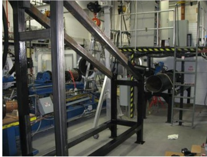
Figure 32. ICES test article support frame and exhaust piping.
