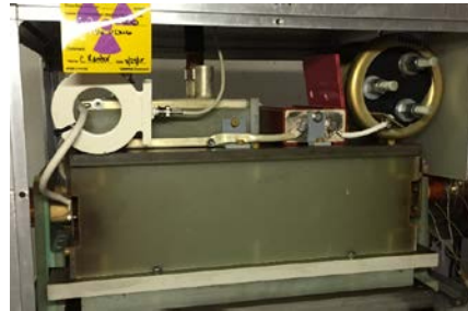
Figure 1: Photo showing free-wheeling diode added to stretch the abort kicker pulse.
