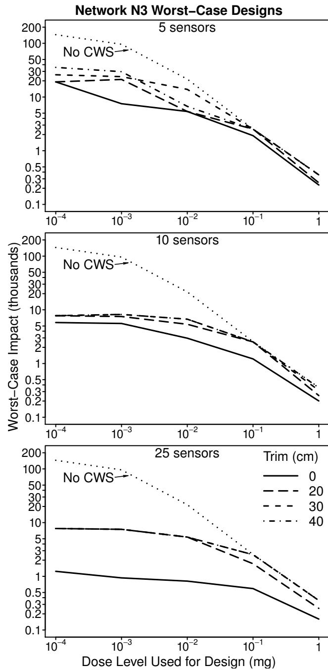
**FIG. 5. Worst-case impact versus dose level for original and transplanted, worst-case CWS designs for Network N3**
