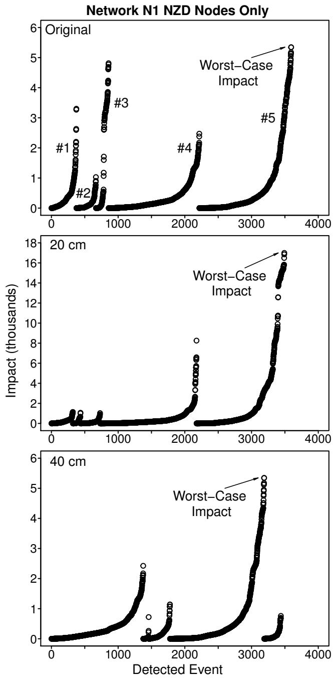
**FIG. 8. Performance of individual sensors for five-sensor, worst-case CWS designs for Network N1 and a dose level of  $10^{-4}$  mg using nonzero demand nodes as possible injection locations**
