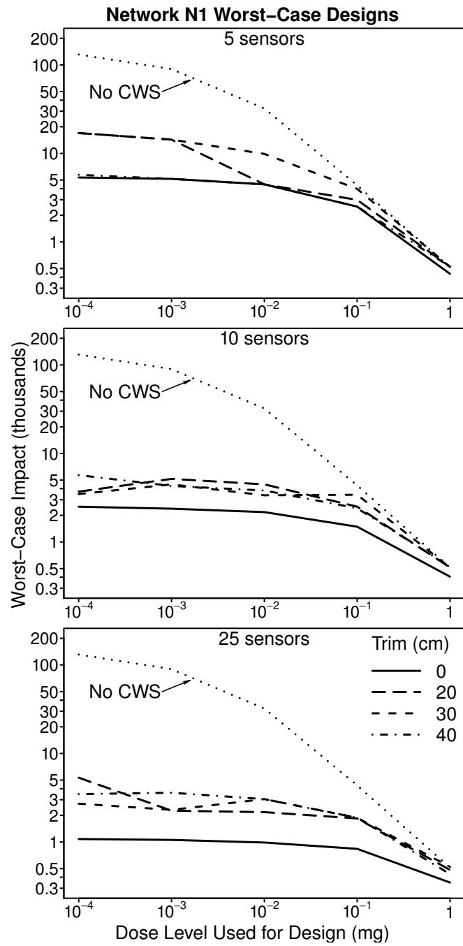
**FIG. 7. Worst-case impact versus dose level for original and transplanted, worst-case CWS designs for Network N1, non-zero demand nodes only**
