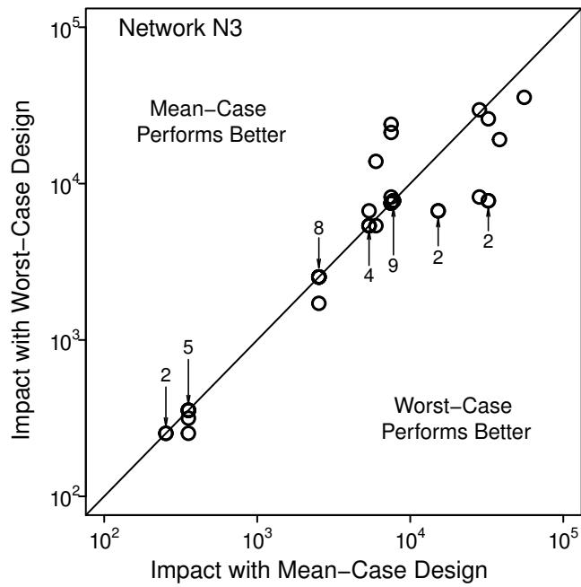
**FIG. 10. Comparison of worst-case impacts for transplanted mean- and worst-case CWS designs, Network N3 (numbers and arrows indicate overlapping or clustered points)**
