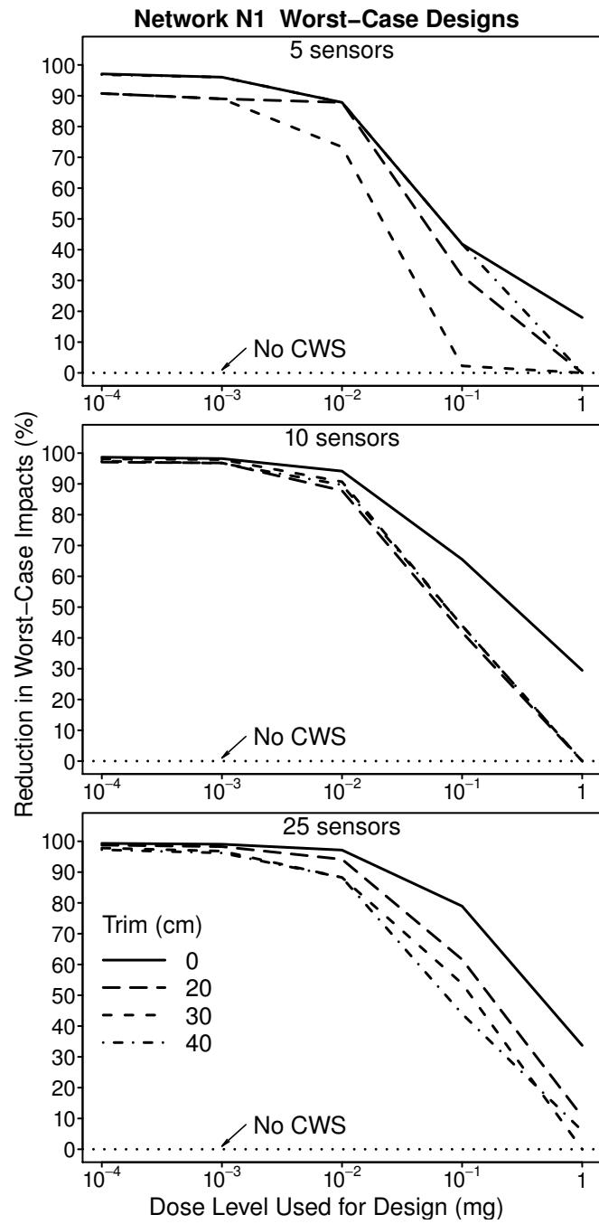
**FIG. 4. Reduction in worst-case impacts obtained with original and transplanted worst-case CWS designs for Network N1 relative to impacts obtained when no CWS is used**
