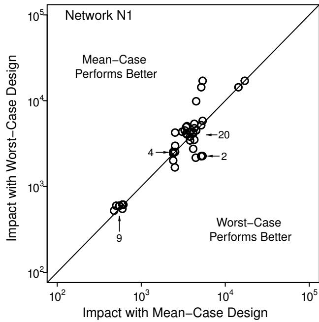
**FIG. 9. Comparison of worst-case impacts for transplanted mean- and worst-case CWS designs, Network N1 (numbers and arrows indicate overlapping or clustered points)**
