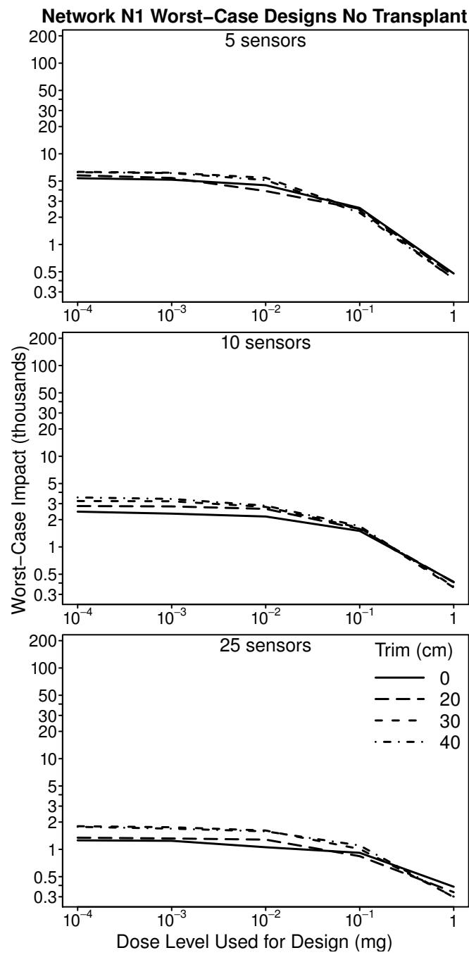
**FIG. 1. Worst-case impact versus dose level for original and non-transplanted, worst-case CWS designs for Network N1**
