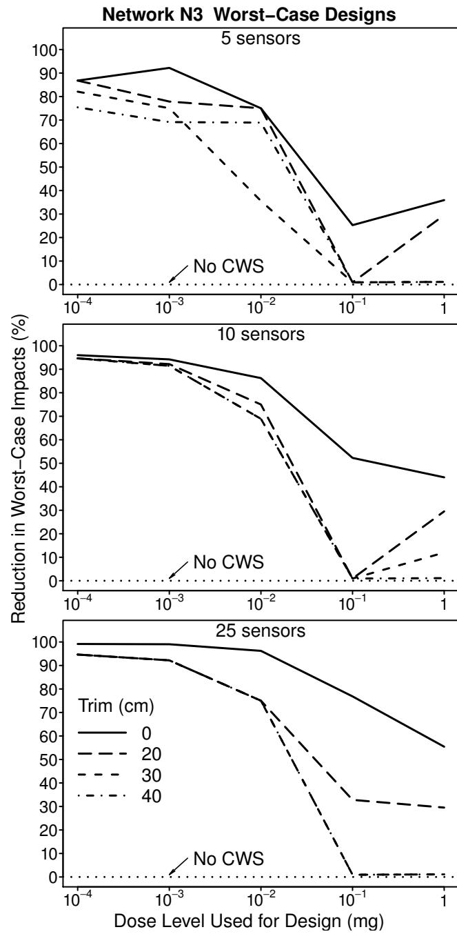
**FIG. 6. Reduction in worst-case impacts obtained with original and transplanted worst-case CWS designs for Network N3 relative to impacts obtained when no CWS is used**
