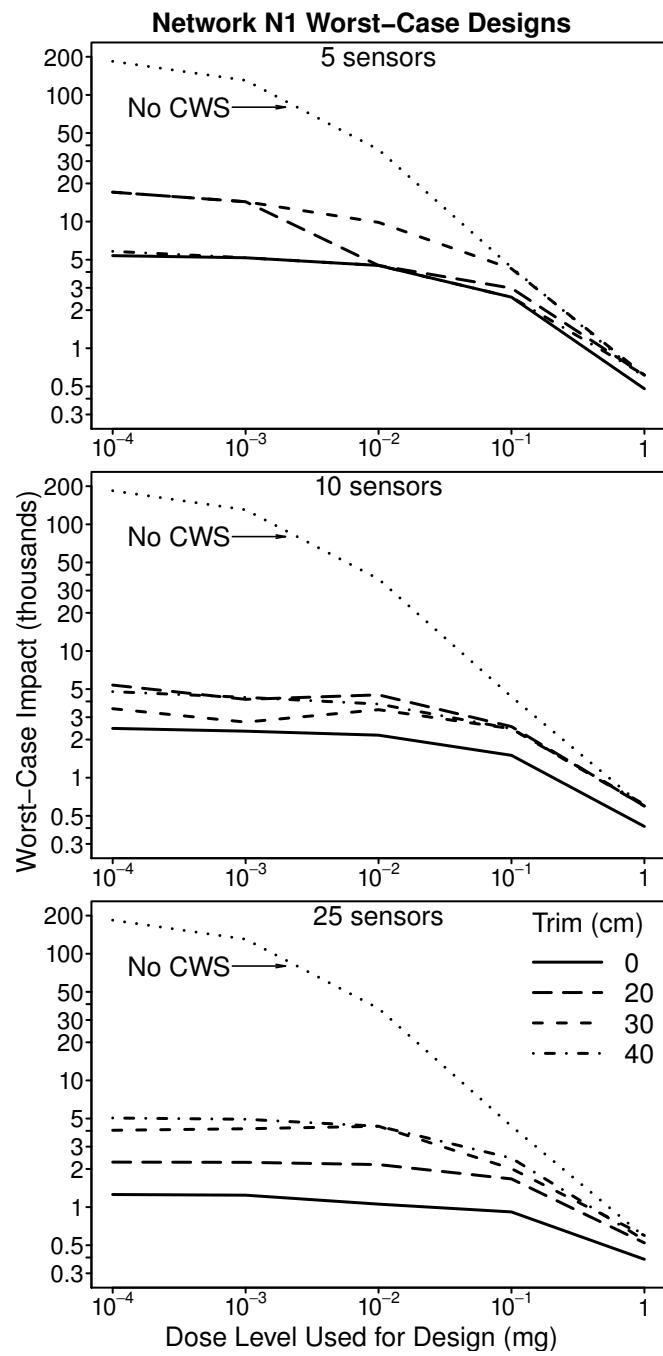
**FIG. 2. Worst-case impact versus dose level for original and transplanted, worst-case CWS designs for Network N1**
