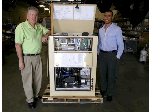
Figure 7 Residential heat pump ready to install.
