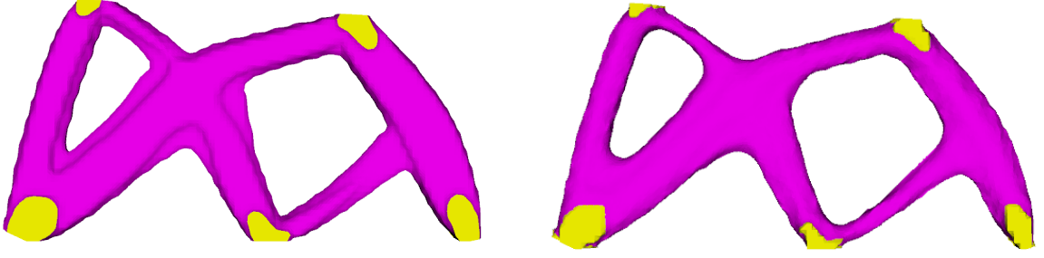
Fig. 2. Left: a full view of the isosurface shown up-close in Fig. 1. Right: The result of removing medium-low frequencies with an implicit method extending the approach of Taubin. The ripples are removed, but so is meaningful geometry! It is very difficult to design polynomial filters that selectively remove narrow frequency bands.
