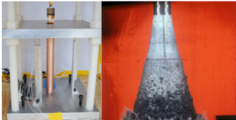
Figure 3 - Cylinder test pre-shot configuration and during detonation (LLNL HE Reference)
