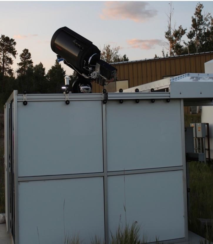
A COTS Raven Class telescope, in this case a 14" Celestron on a Paramount ME tracking mount, is combined with a photon counting sensor to act as a receiver.
