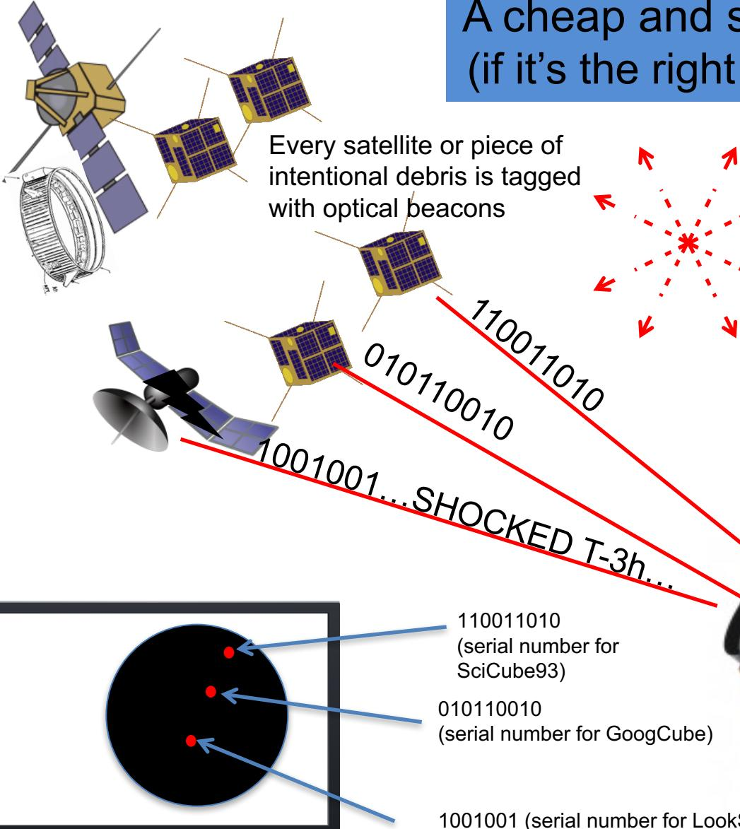
Computer processes x,y to get image of satellites. For each sat, processes times to read the code.
