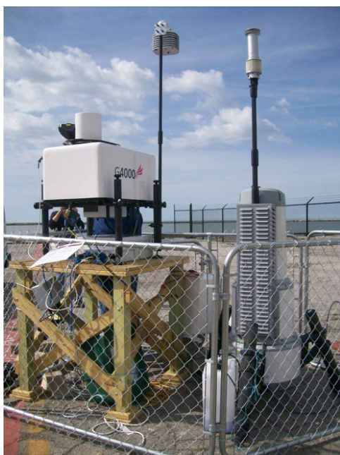
Figure 3.9 Photograph of the scanning doppler lidar (Galion) and vertically pointing lidar deployed at the Port
