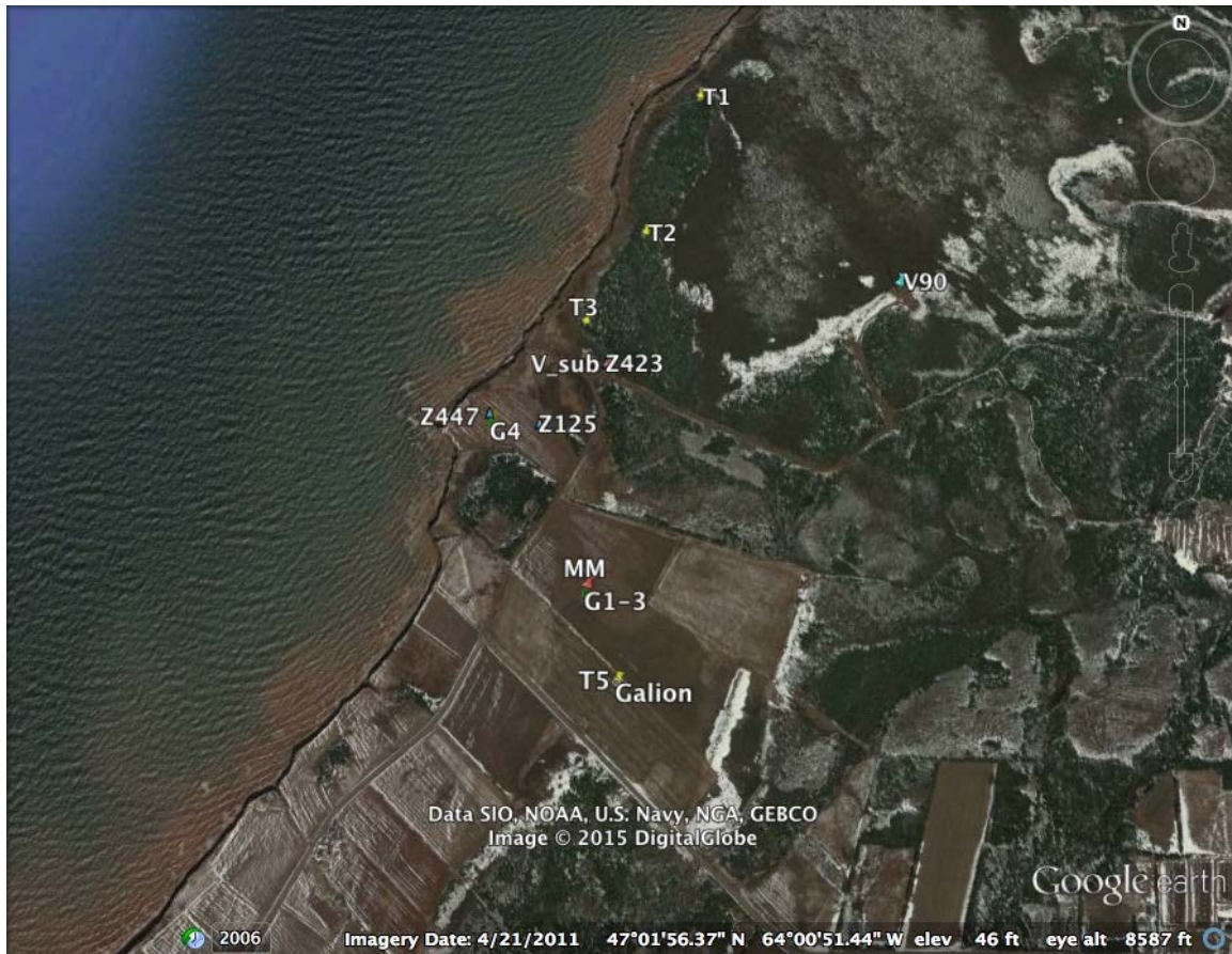
Figure 3.20 Google maps image showing the wind turbines (T1-5), and deployment locations of the 3 ZephIR units (Z125 from WEICan, Z423 and Z447), The meteorological mast (MM) on which three Gill sonic anemometers were deployed (G1-3), the short mast on the coast on which a fourth Gill sonic anemometer was deployed (G4) and the location of the scanning doppler lidar (Galion) that was deployed near the base of T5.
