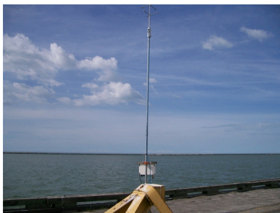
Figure 3.8 Photograph of the Metek sonic anemometer deployed at the Port showing the offshore fetch.
