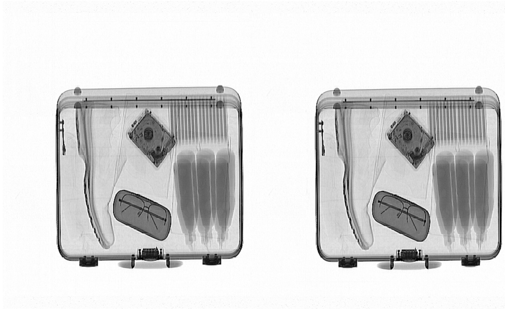
FIGURE 5. Concatenation of the resulting radiographs. The suitcase on the right is offset 1.31 cm from the suitcase on the left.
