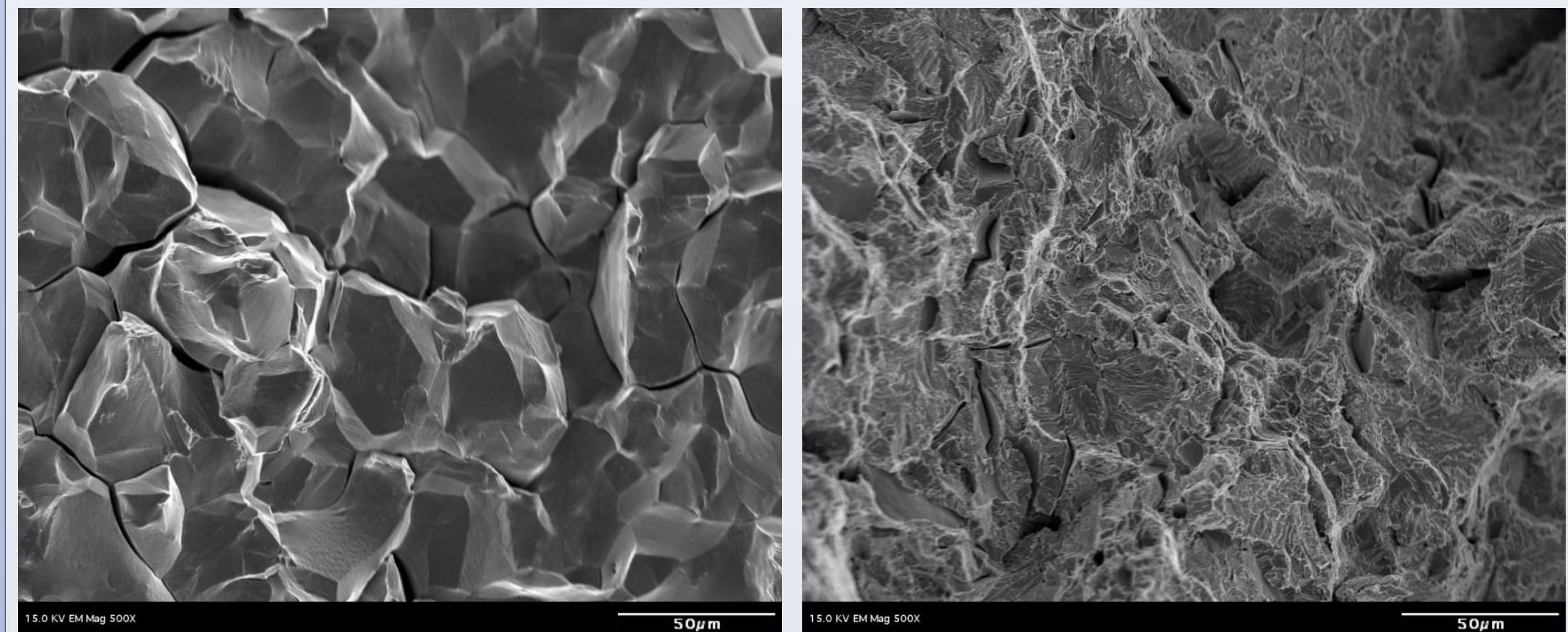
The degree of environmentally-assisted intergranular fracture is reduced by grain-boundary engineering treatments that lead to a large fraction of low-sigma boundaries.
