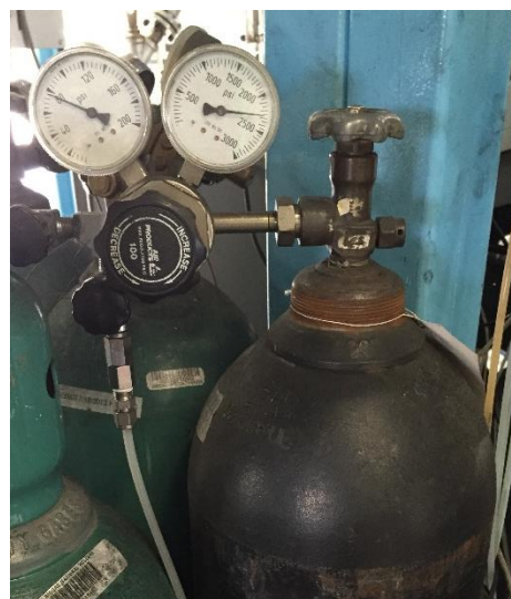
Figure 28. Secondary nitrogen supply
