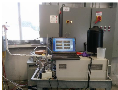
Figure 41. MKS online analyzer connected to BsTU with heat-traced line running from the sample panel.
