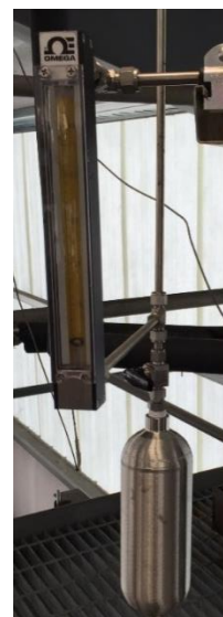
Figure 33. HX-310 condensate collection vessel.
