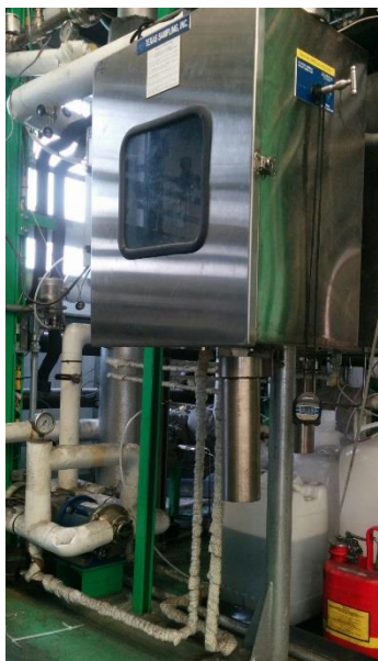
Figure 37. Heat-traced sample lines running to and from liquid sampling box.
