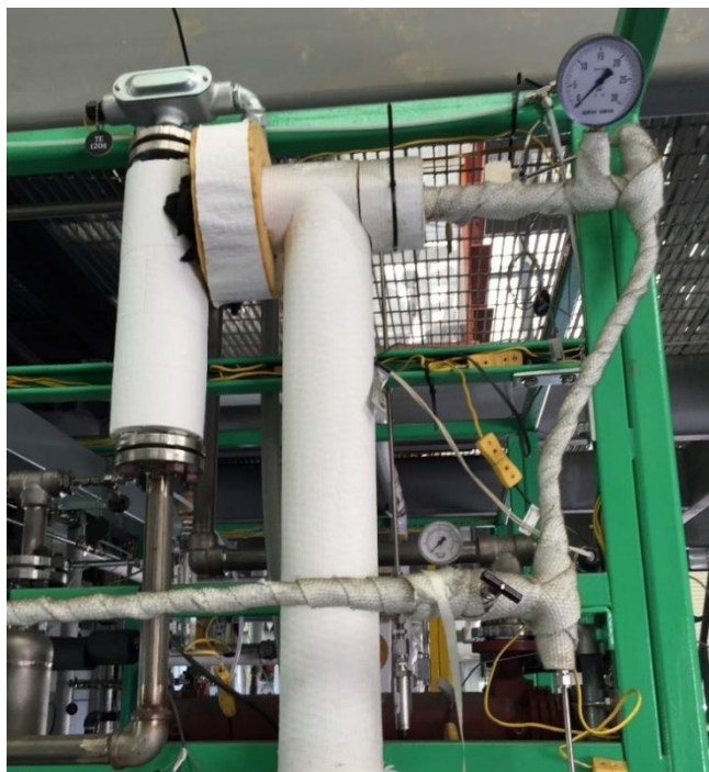
Figure 30: Steam injection system for humidifying feed gas through an orifice plate, right, and HX-120, left.
