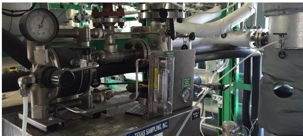
Figure 29: Solvent addition system with diaphragm pump, left, and absorber sump, right.
