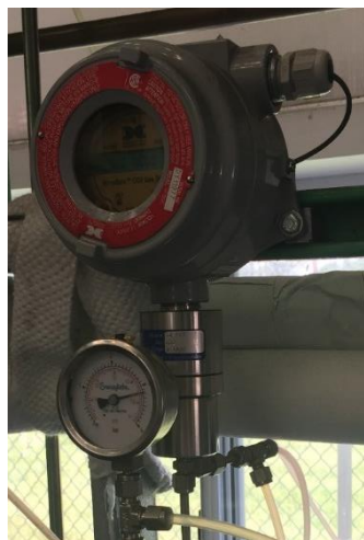
Figure 39. DETCON CO 2 analyzer added to the regenerator effluent
