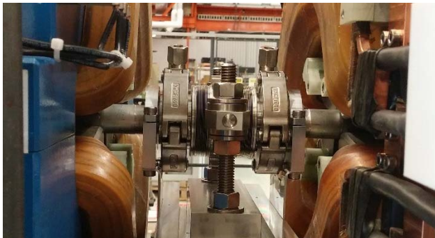
Figure 3: Mock-up BPM in an integrated test assembly.
