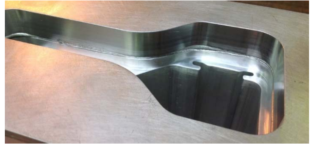
Figure 4: Automated 2 mm thick aluminium profile weld.
