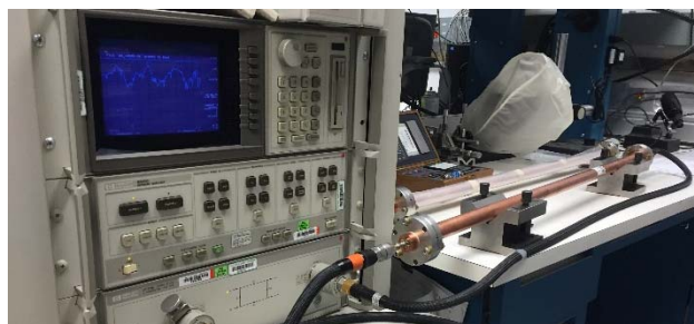
Figure 6: Network analyzer measurements on a copper vacuum chamber prior to NEG coating.
