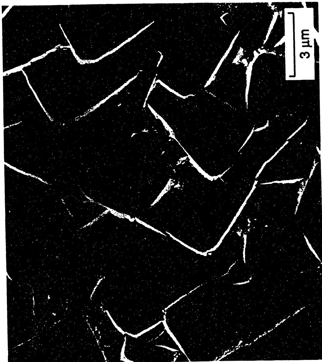
The grains contain no twins or stacking faults
