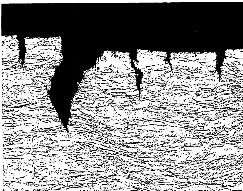
Figure F.3 Photomicrograph Of SSR Specimen Of Alloy CDA 102 Exposed To 0.005M NaNO 2 At 23°C And Polarized To +0.200 Volts (SCE). Specimen Strained To Failure At 1 \times 10^{-6} \text{ sec}^{-1} ; 100X Magnification (Test No. 19).
