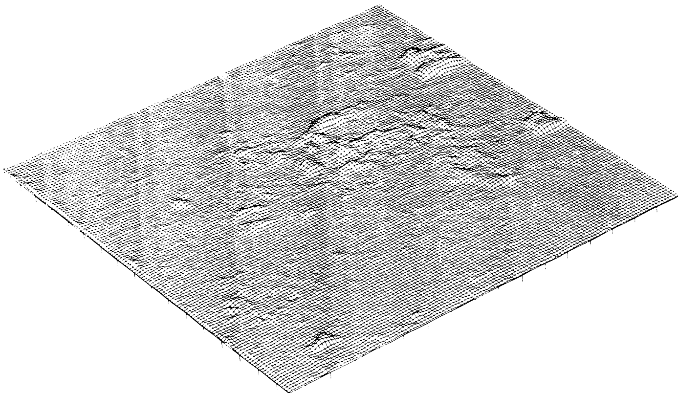
Figure 2. Aperture surface measured by casting-and-imaging technique (C1). [XBL 896-2198]
