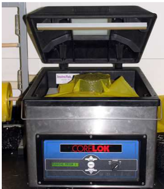
Figure 4.2: CoreLok apparatus with sealed sample
