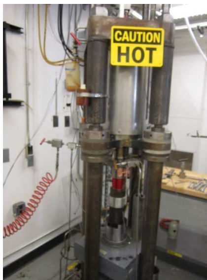
Figure 3.3 – Photograph of creep load frame in the SNL Geomechanics Laboratory with pressure vessel (steel cylinder directly behind caution sign).
