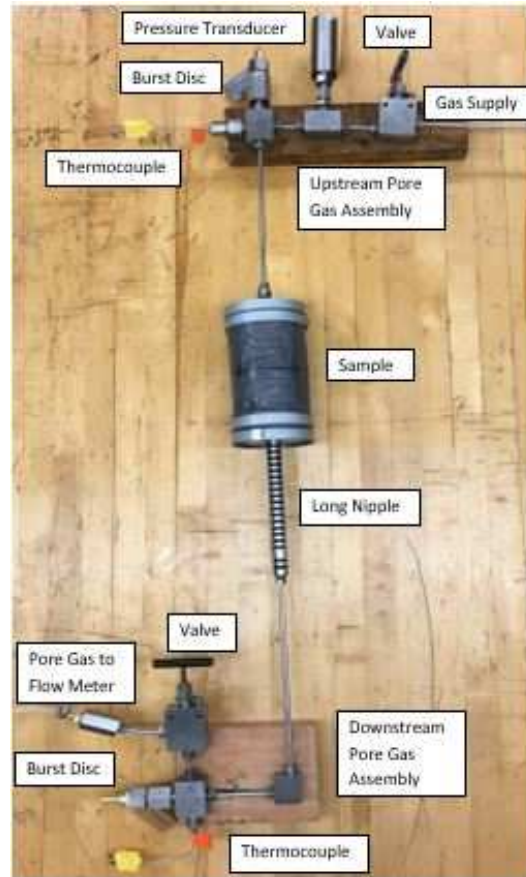
Figure 3.7 – Pore gas line assembly showing current configuration
