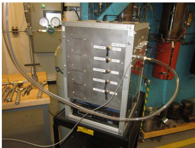
Figure 3.5 - Flow bench used to measure steady state flow rates during constant pressure gas flow tests.
