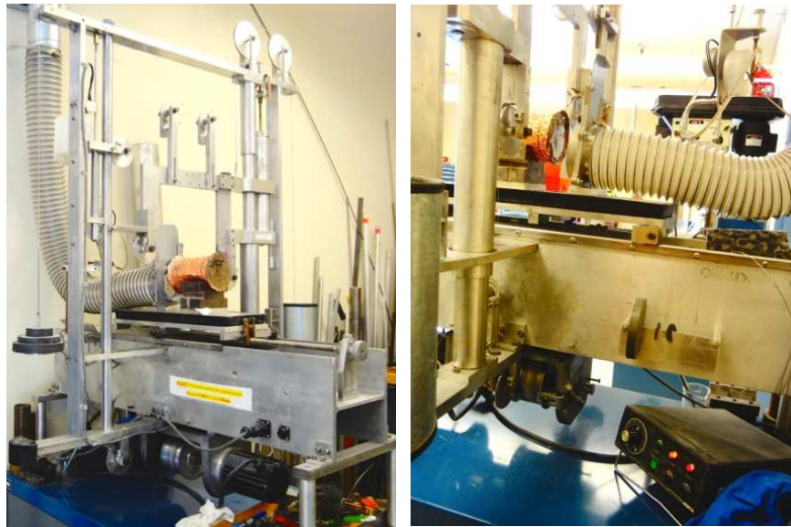
Figure 5.5: Diamond wire saw with ventilation, pulley system, adjustable table, wheel, pump and pump controller.
