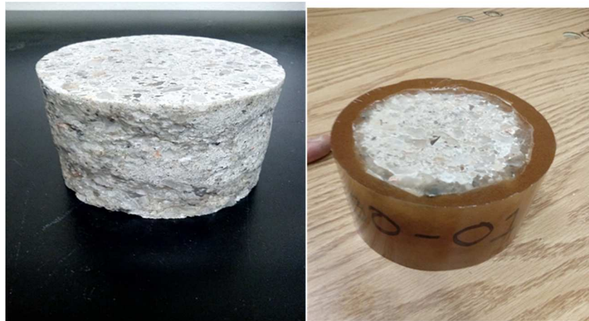
Figure 4.1 – Central core of post-consolidated sample prior to (left) and after being cast in epoxy (right).
