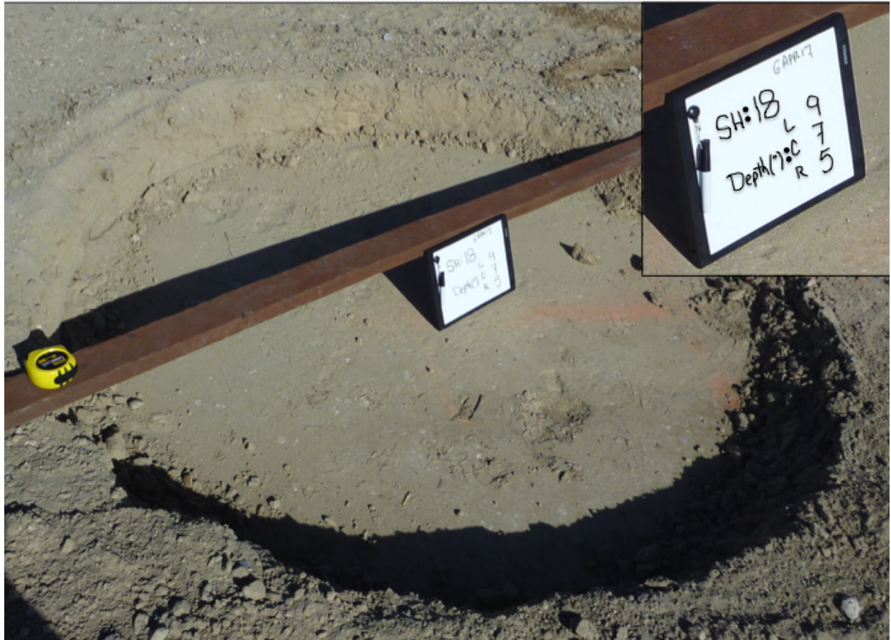
Figure 3. Example of depression left after successive hits in shot location 18. Here the ground compacted more to one side. See Figure 2 for location.
