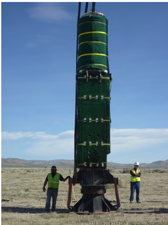
Figure 1. The 13,000 kg Seismic Hammer™
