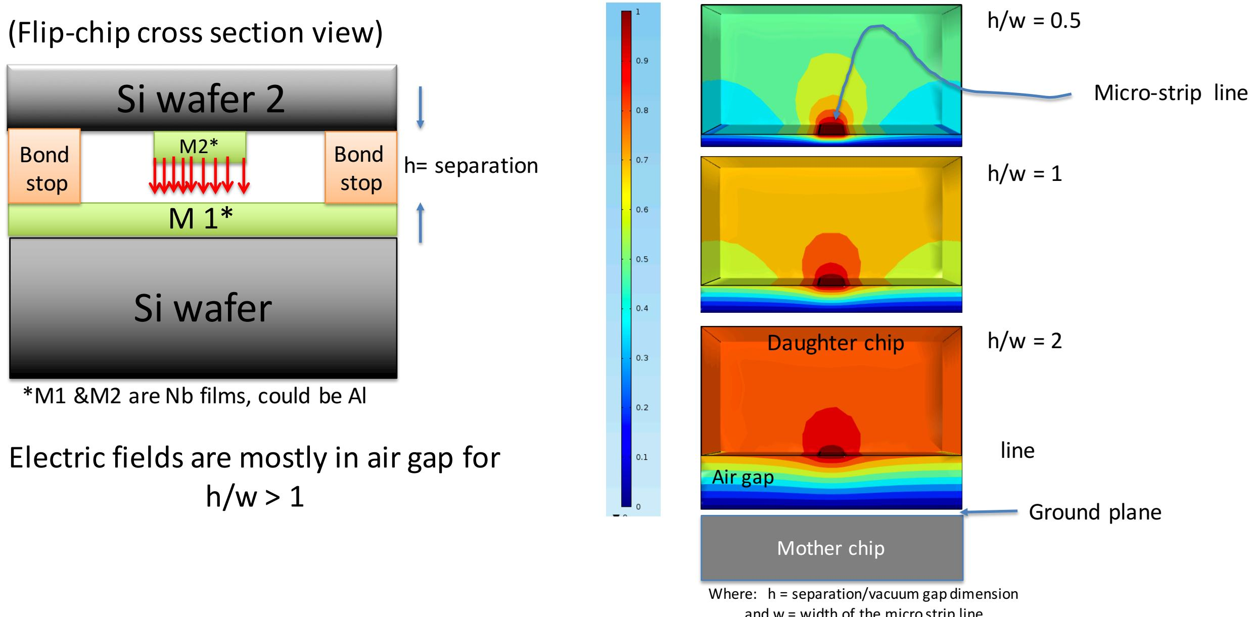
Electric fields are mostly in air gap for  $h/w > 1$
