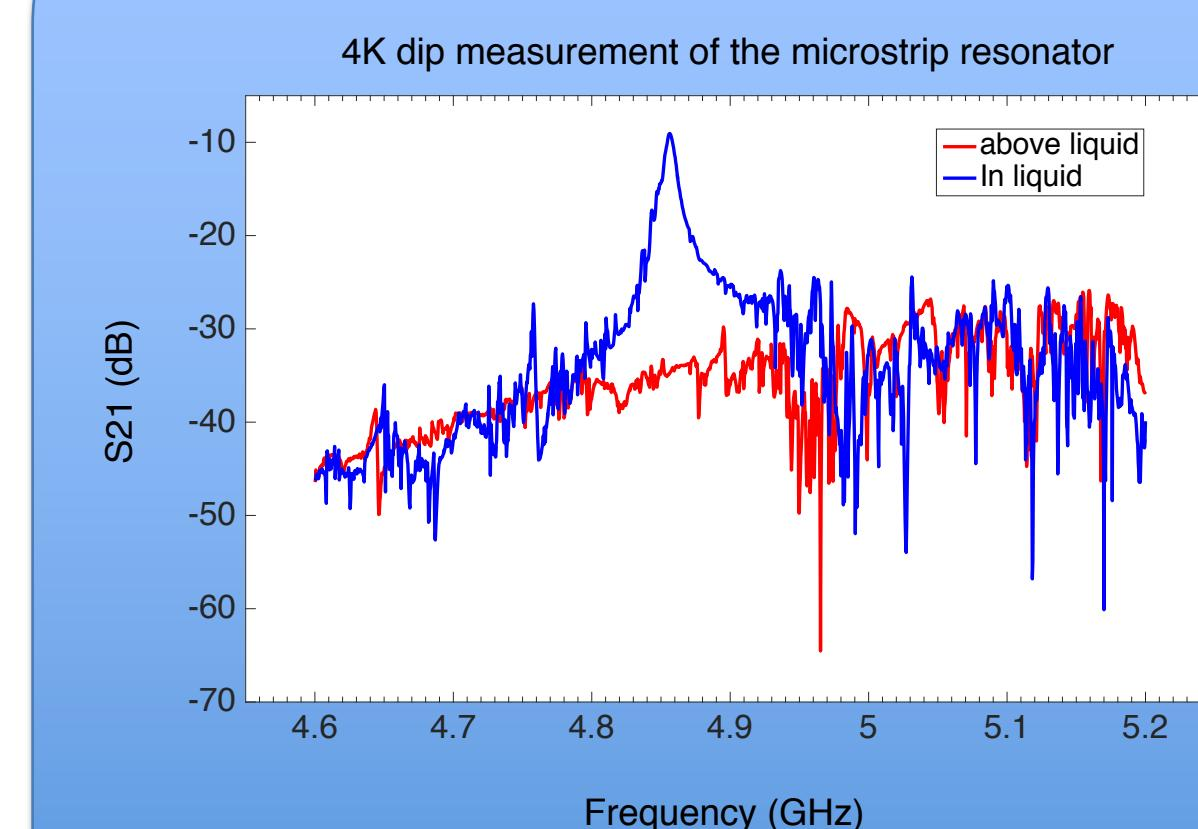
4K dip measurement of the microstrip resonator
